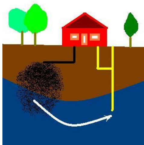
Fig. 1. Contaminated groundwater from septic systems
