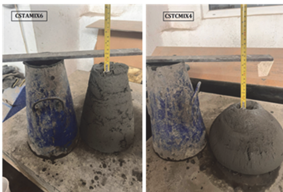
Fig. 6. The slump method for experimental eco-concrete 3D printing samples
