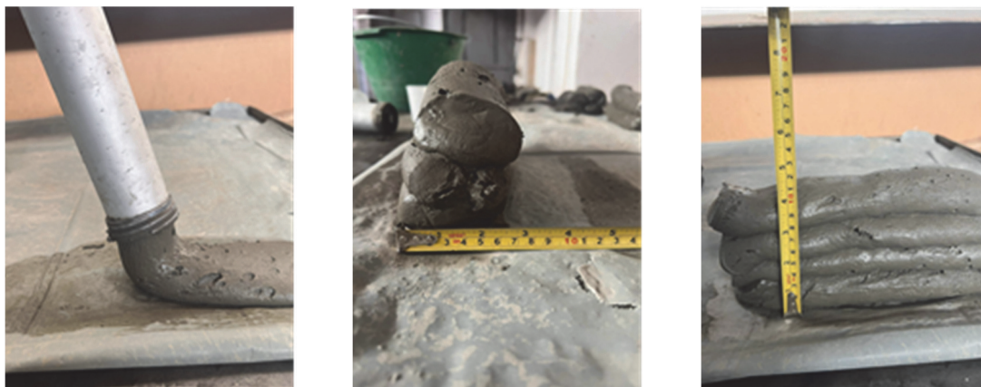
Fig. 3. Printing process- extruded filament (left), shape stability (middle) multi-layer’s structure (right)
