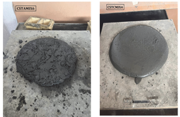
Fig. 8. Jump table method for experimental eco-concrete 3D printing samples
