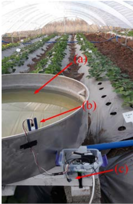
Fig. 2. The data collection unit inside the greenhouse. (a) evaporation pan, (b) water level sensor, and (c) environmental sensor
