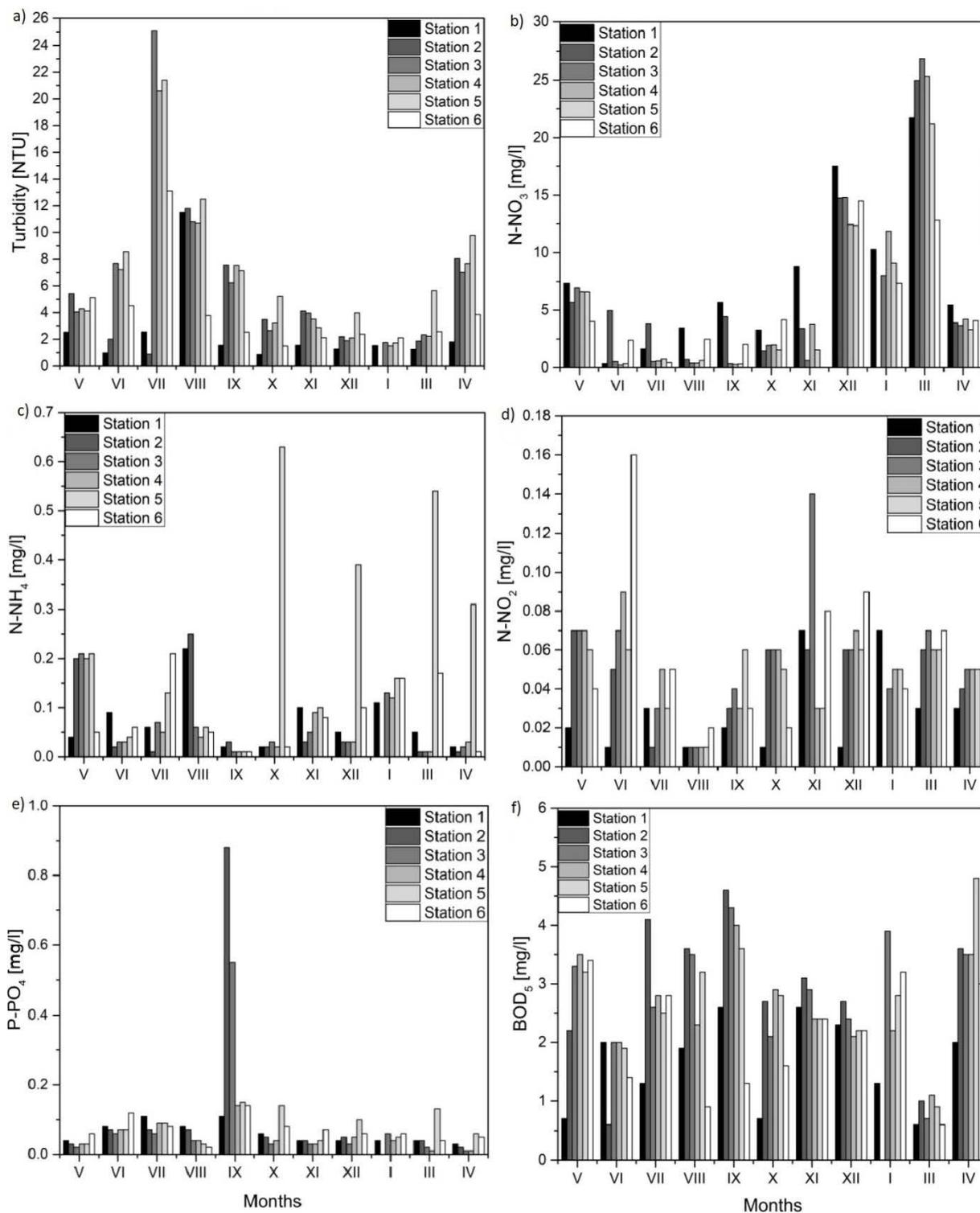
Fig. 6. (a)-(f) Monthly values of selected physicochemical parameters at the sampling stations in the Michallice Reservoir, May 2016 – April 2017
