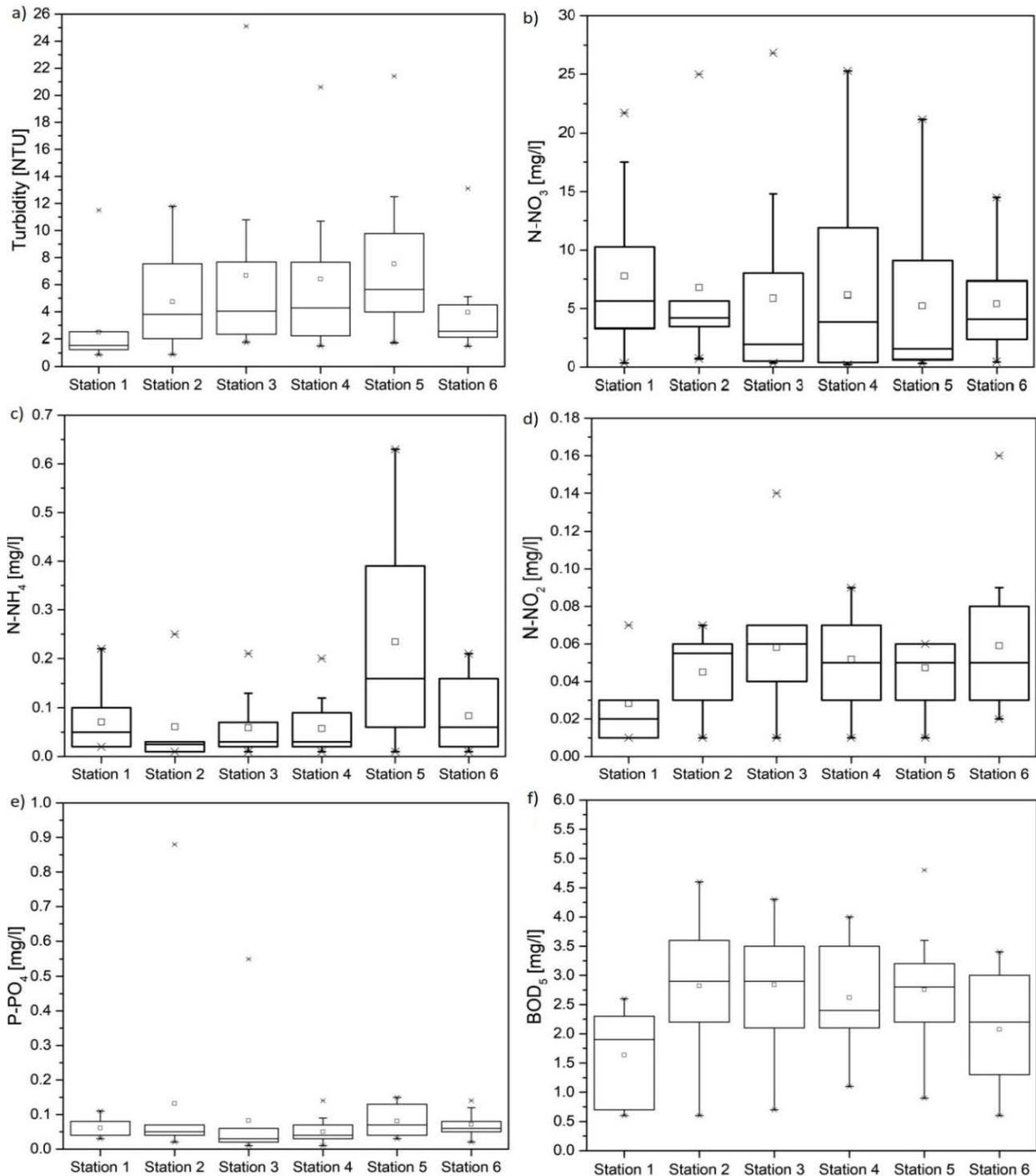
**Fig. 7.** (a)-(f) Boxplots of selected physicochemical parameters at the sampling stations in the Michallice Reservoir, May 2016 – April 2017
