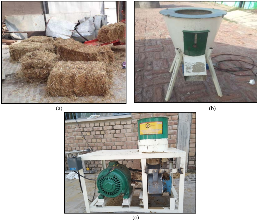
Fig. 1. Materials and machines used for the experiments: (a) represents cuboidal straw bales, (b) depicts the leaf shredder; (c) shows the pellet machine
