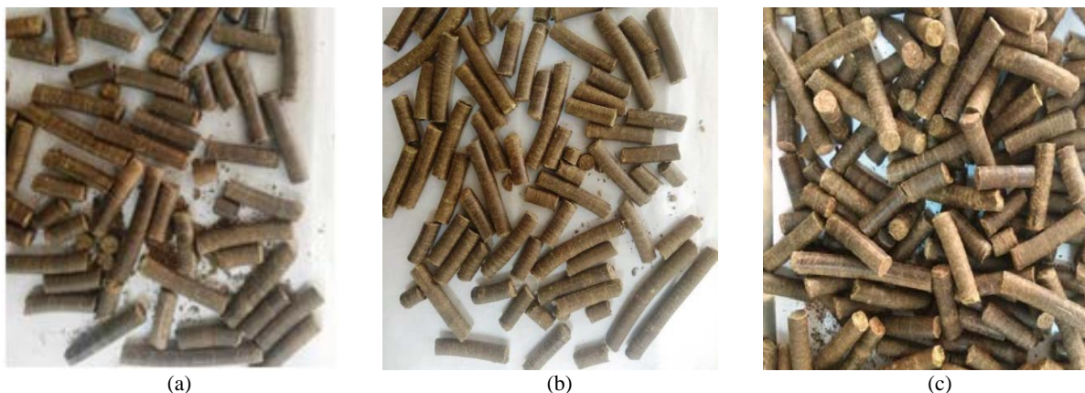
Fig. 4. Pellets made using different ratio of PS and SD (a) 50:50 (b) 80:20 (c): 100:0
