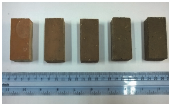
Fig. 5. Colours of laboratory-made ceramic bodies made (ceramic bodies from right to left: TS2.5, TS5, TS10, TS15)
