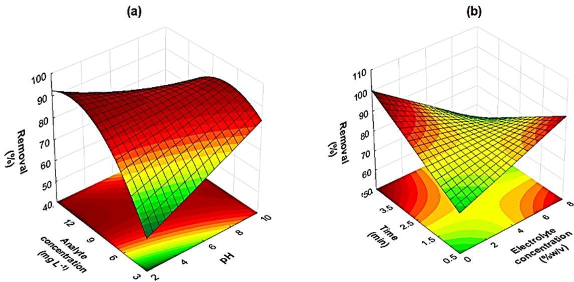
**Fig. 4.** Response surface plots for the methylene blue removal: (a) Analyte concentration–pH; (b) Time–electrolyte concentration
