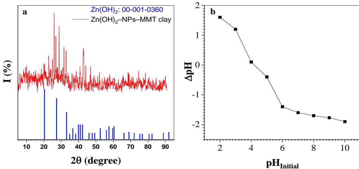
Fig. 3. a. XRD pattern of the  $\text{Zn(OH)}_2$ -NPs-MMT clay; b.  $\text{pH}_{\text{pzc}}$  values of  $\text{Zn(OH)}_2$ -NPs-MMT clay. Condition:  $\text{Zn(OH)}_2$ -NPs-MMT clay 0.1 g; sample volume 50 mL; supporting electrolyte  $\text{KNO}_3$  0.1 mol  $\text{L}^{-1}$ ; stirred time: 24 h
