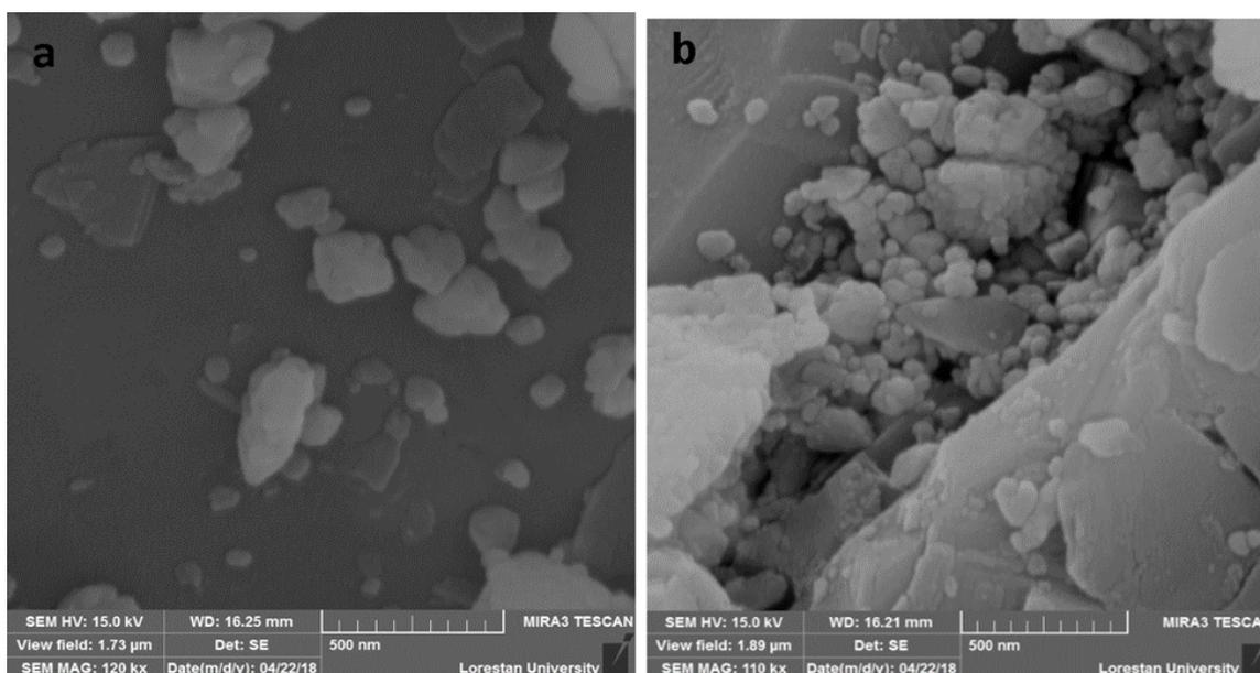
Fig 1. SEM micrograph of a natural clay and b Zn(OH)<sub>2</sub>–NPs–MMT clay
