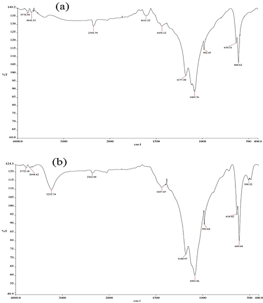
Fig. 2. FTIR spectra of (a) natural clay and (b)  $\text{Zn(OH)}_2$ -NPs-MMT clay
