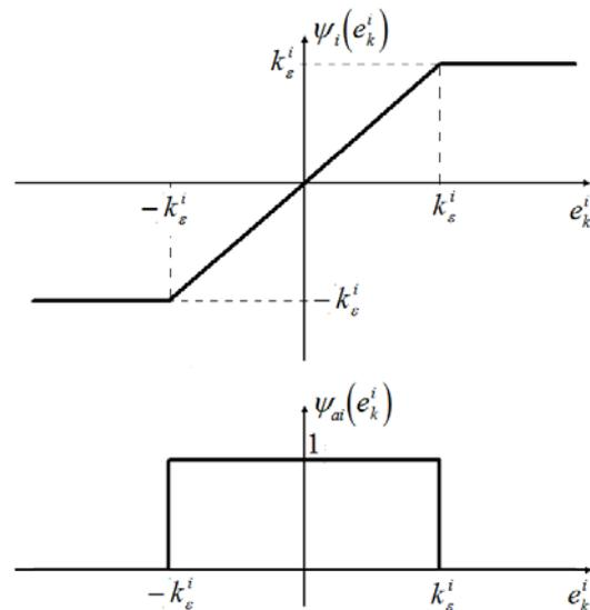
Fig. 4. Huber's function and approximation of the first derivative of the pseudo-Huber's function
