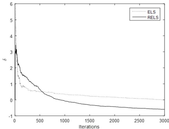
Fig. 9. Comparison of extended least squares (ELS) and robust extended least squares (RELS) for  $\sigma = 0.15$
