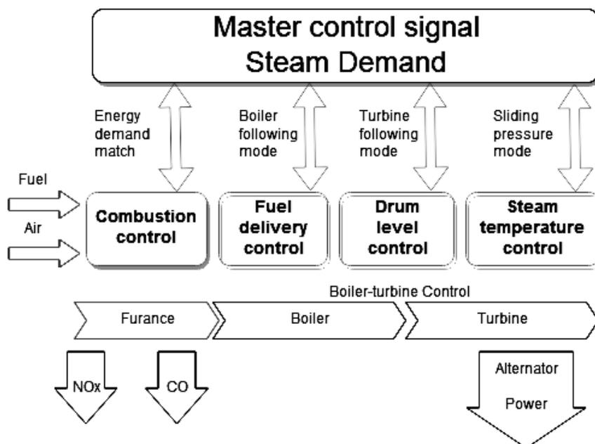
Fig. 1. Control of the traditional thermal power plant
