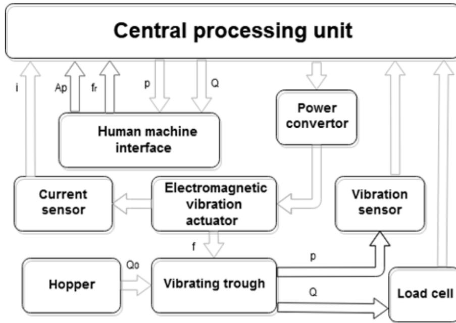
Fig. 2. Control of the vibratory conveyor with an electromagnetic actuator
