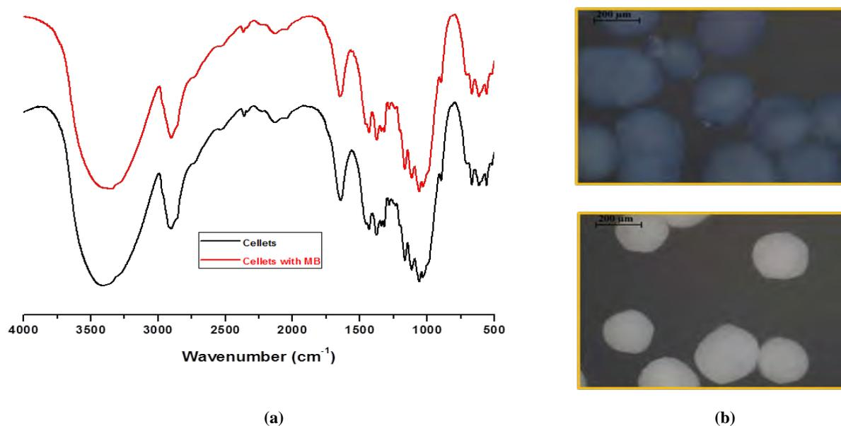
Fig. 1. FTIR spectra (a) and PLM microphotographs (b) of *Cellets 200* before and after adsorption
