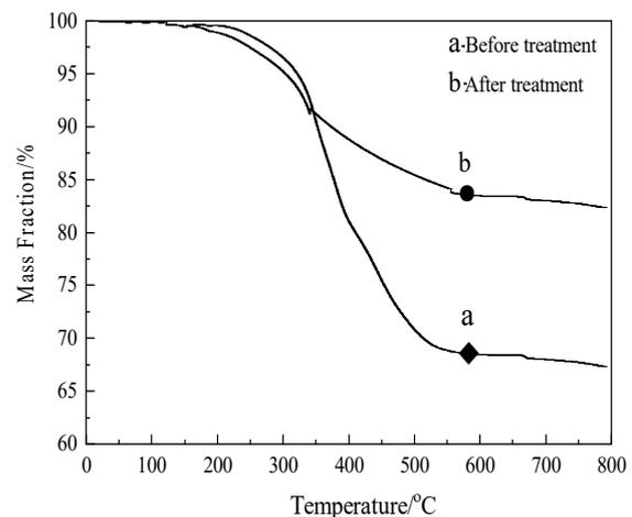
Fig. 9. TG curve of oily sludge
