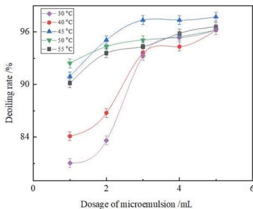
Fig. 8. Relationship between micro-emulsion dosage, treatment temperature, and deoiling rate
