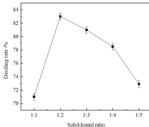
**Fig. 6.** Deoiling rate of oily sludge under different solid-liquid ratios
