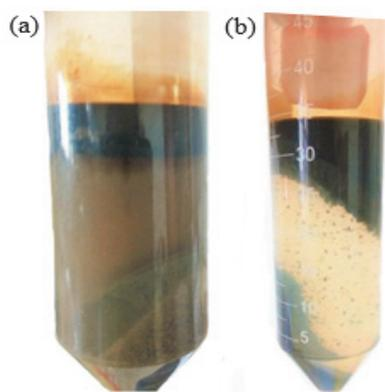
**Fig. 5.** Effects of different micro-emulsions on: (a) Other micro-emulsion treatment of oily sludge, and (b) No.1-5 micro-emulsion treatments of oily sludge
