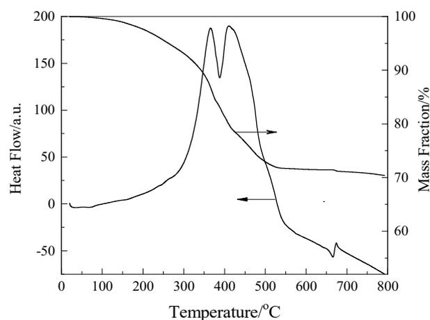
Fig. 3. TG/DTA spectrum of oily sludge
