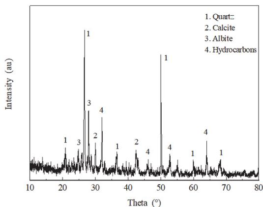
Fig. 2. XRD spectrum of oily sludge
