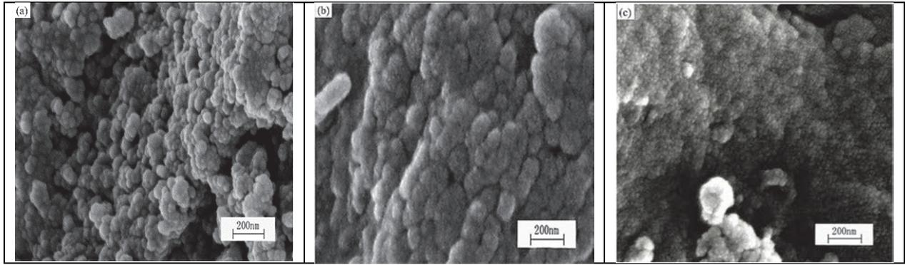
**Fig. 10.** SEM images of oily sludge with (a) No micro-emulsion added, (b) Micro-emulsion added and (c) Treatment with quenching and tempering centrifugation with micro-emulsion
