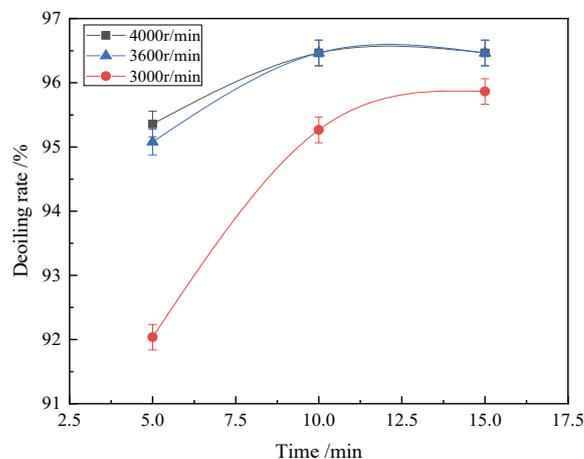
**Fig. 7.** Relationship between centrifugation speed and centrifugation period
