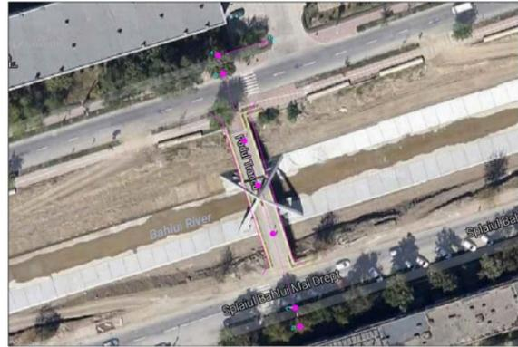
**Fig. 7.** Trigonometric levelling network
