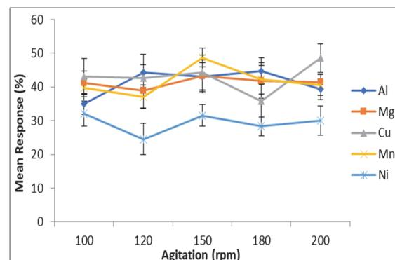
**Fig. 6.** Effects of Agitation on mean responses for metal ions dissolution
