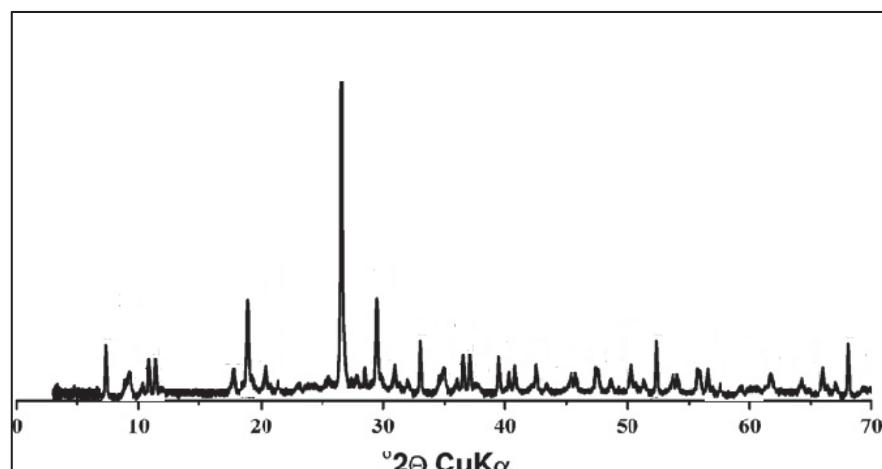
**Fig. 1.** X-Ray diffractogram of brown shale ore
