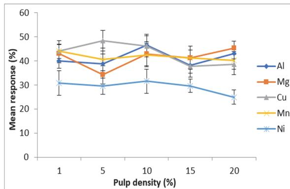
**Fig. 4.** Effects of pulp density mean responses for metal ions dissolution
