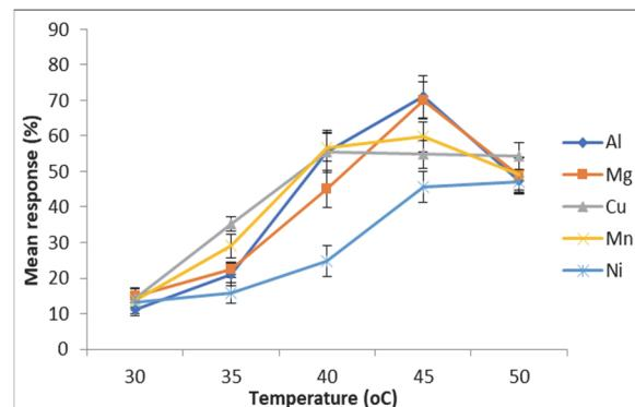
**Fig. 5.** Effects of temperature on mean responses for metal ions dissolution
