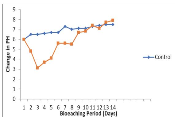
**Fig. 7.** pH changes during metals bio recovery studies. All values are means of duplicates with an error of  $\pm 0.05$
