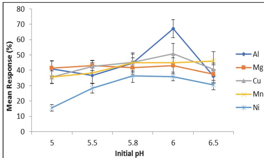
**Fig. 2.** Effects of Initial pH on mean responses for metal ions dissolution
