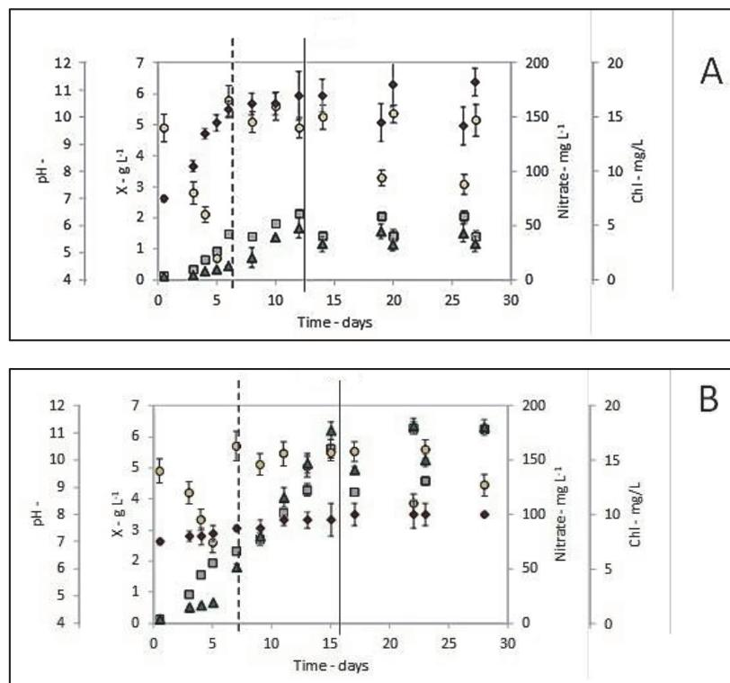
**Fig. 2.** Cultures of *G. emersonii* at different operating conditions: (A) represents the culture with only air sparged while (B) represents the culture with CO<sub>2</sub> added. Dashed lines mark the beginning of fed-batch state. Continuous lines mark the beginning of semicontinuous mode. Biomass concentration [X] was indicated by squares. Chlorophyll a concentration was indicated by triangles. pH was indicated by rhombus. Nitrate concentration was indicated by circles
