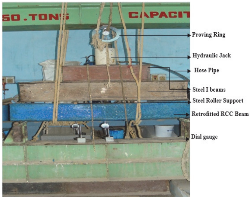
Fig. 3. Laboratory experimental beam-loading set-up
