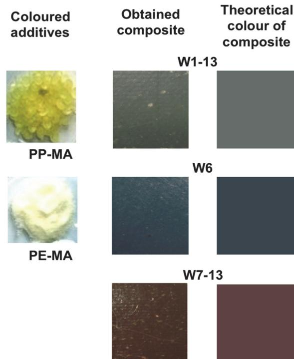
**Fig. 5.** Actual and predicted color of the MSW composites**Table 2.** CIELAB color parameters of the polymer composites
