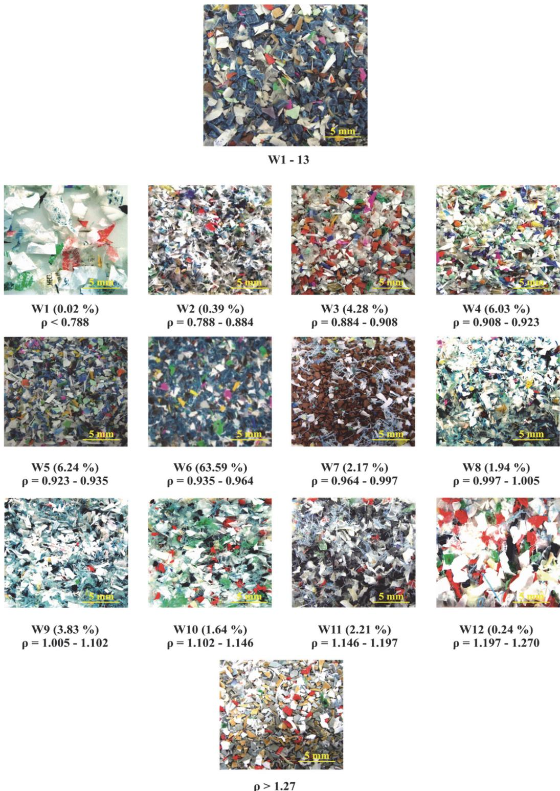
**Fig. 1.** MSW wastes separated in density fractions by the flotation method (density units: g/cm<sup>3</sup>)
