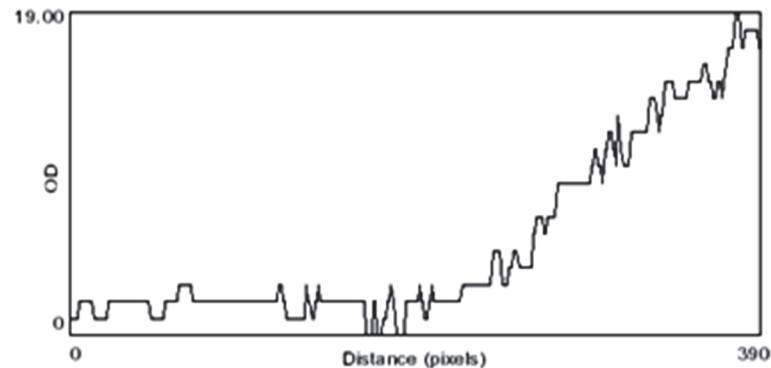
**Fig. 6.** The variation in the contrast of the image (expressed in optical density units)
