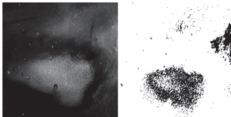
**Fig. 11.** The aerosol particles on a lamella, at floor level –left and the related distribution of the sample particles -right.
