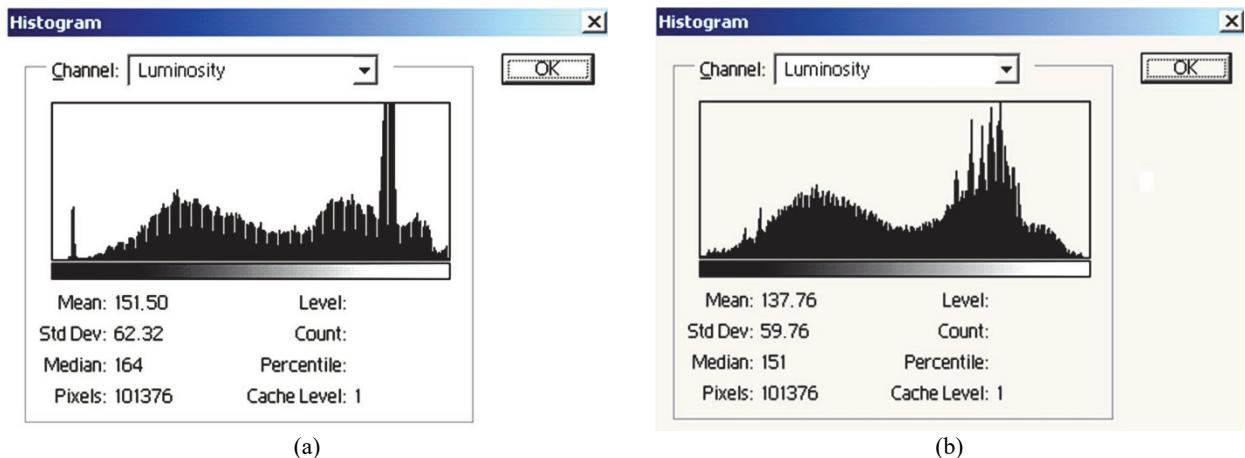
**Fig. 7.** The histograms of an image acquired and of a calibrated image: (a). The histogram of an image acquired converted into gray levels (8-bit); (b). Calibrated image histogram
