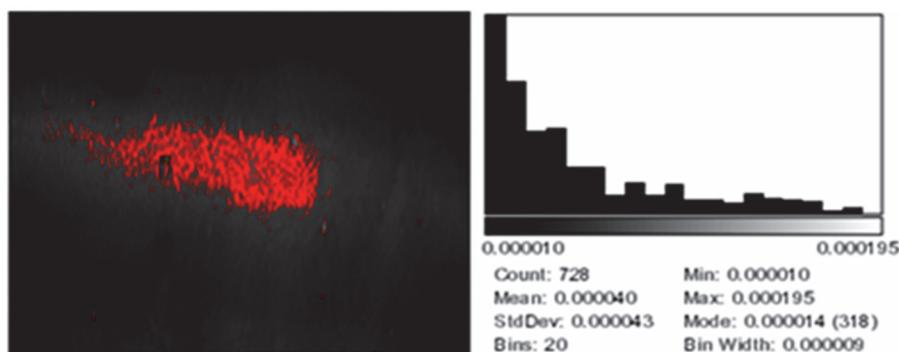
**Fig. 10.** The limitation of the interest area through software –left and related distribution of particles-right
