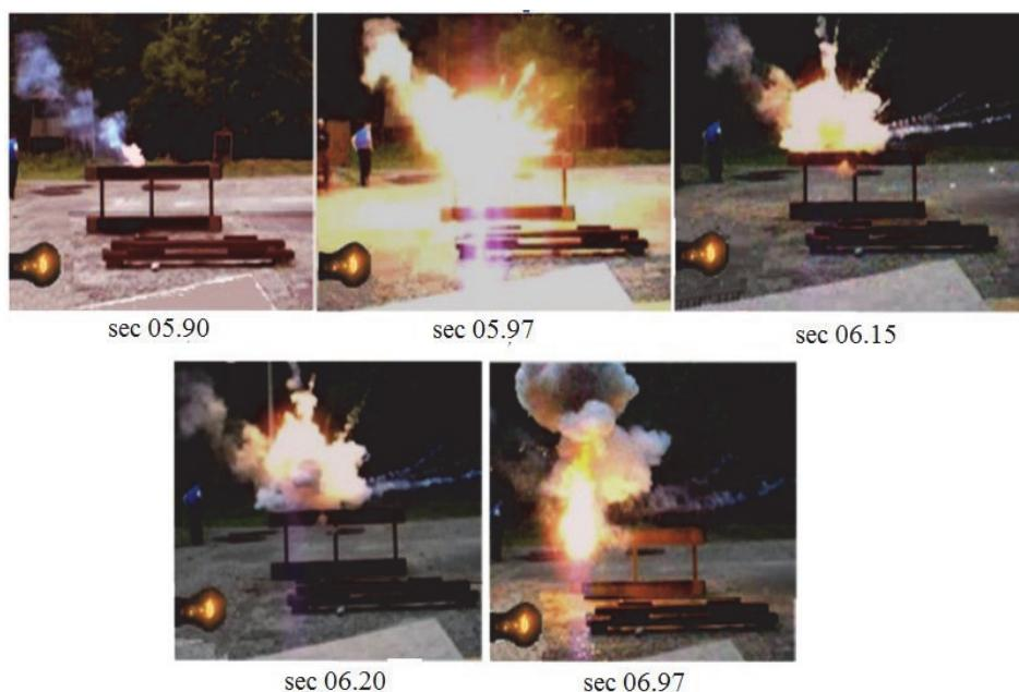
**Fig. 1.** An explosion dynamics as viewed in visible spectrum (pyrotechnic produced aerosol)
