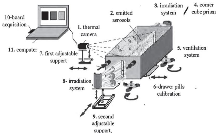
**Fig. 3.** Principle of the used experimental system using IR- thermovision equipment, where: 1-is thermal camera, 2-emitted aerosols, 3 (8)- irradiation system doubled, 4- corner cube prism, 5-ventilation system, 6-drawer pills calibration, 7 first adjustable support, 8- irradiation system, 9-second adjustable support, 10-board acquisition and 11-computer)
