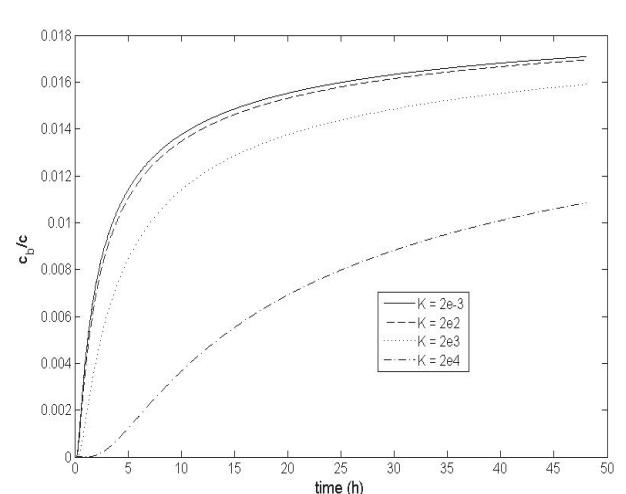
**Fig. 9.** Dependency of the surface dye concentration on the different values of the sticking coefficient ( $K$ ), the value used for the calculations are  $D_0 = 2 \times 10^3$ ,  $c = 6 \times 10^{21} \text{ m}^{-3}$ ,  $l_{mol} = 0.5 \times 10^{-9} \text{ m}$ ,  $\Gamma_{max} = 5 \times 10^{19} \text{ m}^{-2}$  and  $d = 13 \mu\text{m}$
