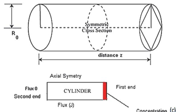
**Fig. 2.** Illustration for model setup and boundary conditions
