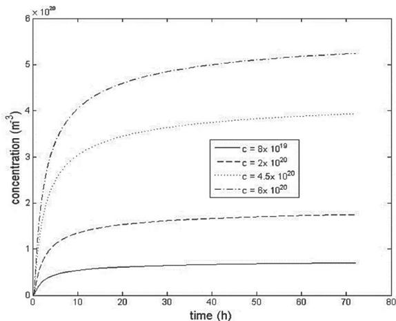
**Fig. 3.** Dependency of the surface concentration on the different values of the initial dye concentration ( $c$ ), the value used for the calculations are  $k = 2 \times 10^3$ ,  $D_0 = 5 \times 10^{-9} \text{ m}^2 \text{s}^{-1}$ ,  $l_{\text{mol}} = 0.5 \times 10^{-9} \text{ m}$ ,  $\Gamma_{\max} = 5 \times 10^{19} \text{ m}^{-2}$  and  $d = 13 \mu\text{m}$  is the length of the film
