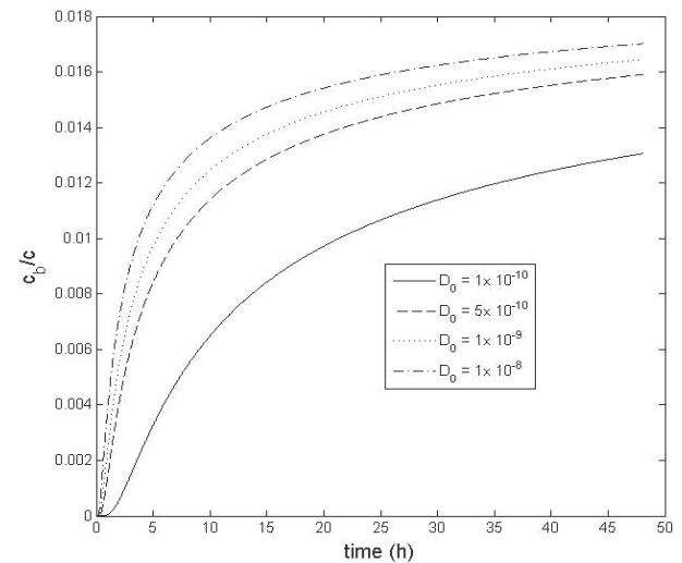
**Fig. 8.** Dependency of the surface dye concentration on the different values of the diffusion coefficient ( $D_0$ ), the value used for the calculations are  $K = 2 \times 10^3$ ,  $c = 6 \times 10^{21} \text{ m}^{-3}$ ,  $l_{mol} = 0.5 \times 10^{-9} \text{ m}$ ,  $\Gamma_{max} = 5 \times 10^{19} \text{ m}^{-2}$  and  $d = 13 \mu\text{m}$
