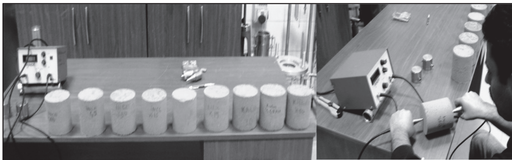
Fig. 2. Ultrasonic test of compacted samples
