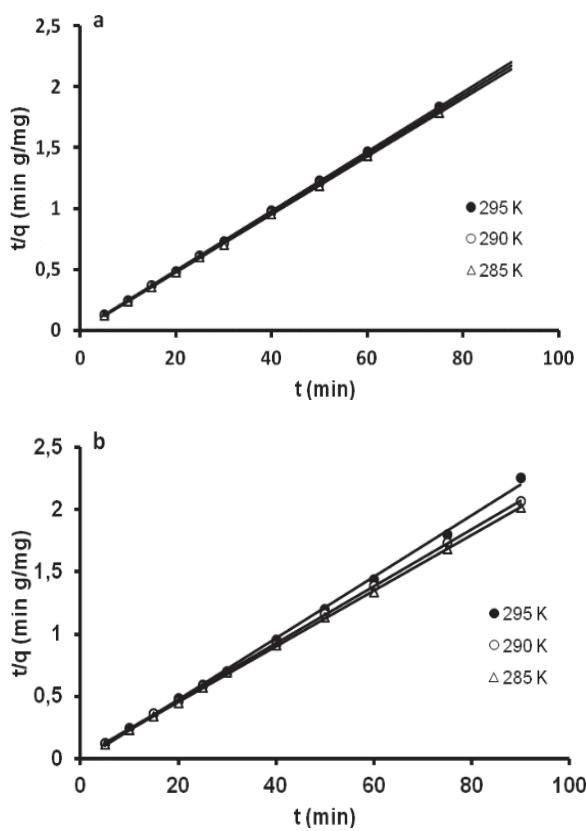
**Fig. 7.** The best fit of the pseudo-second order kinetic equation (Eq. (4)) for Cu(II) adsorption by lyophilized cells of (a) *P. aeruginosa* and (b) *P. fluorescens* at temperatures 285, 290 and 295 K
