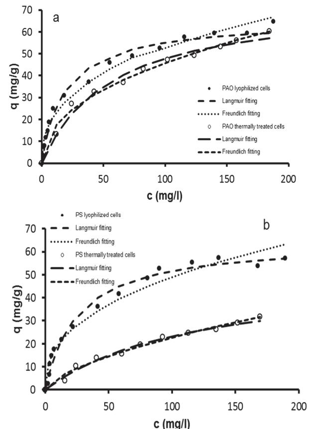
**Fig. 8.** Bioadsorption isotherms of lyophilized and thermally inactivated cells of (a) *P. aeruginosa* (PAO) and (b) *P. fluorescens* (PS) for Cu(II) ions in the initial Cu(II) concentration range of 5–250 mg/L (biomass concentration: 1 g/L, pH = 5.4, temperature: 285 K)
