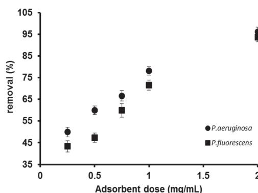
**Fig. 6.** Effect of the biosorbent dose on the Cu(II) uptake by *P. aeruginosa* and *P. fluorescens* biomass.
