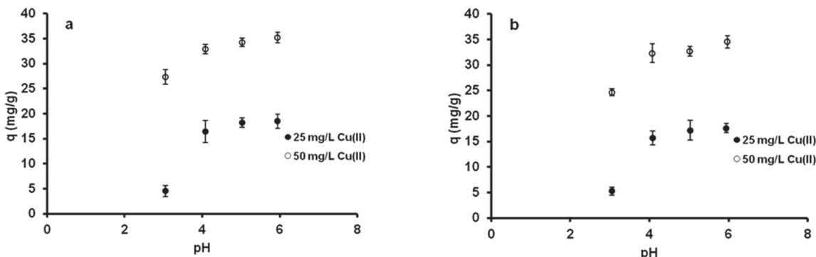
Fig. 4. Effect of pH on the adsorbed Cu(II) amount ( $q$ ) on: (a) *P. aeruginosa* and (b) *P. fluorescens* biomass
