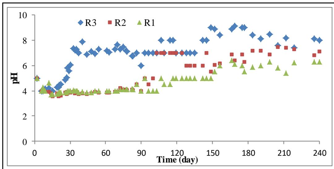
**Fig. 3.** The variation of pH profile of leachate from R1, R2, and R3 hybrid anaerobic–aerobic bioreactors during the operation time
