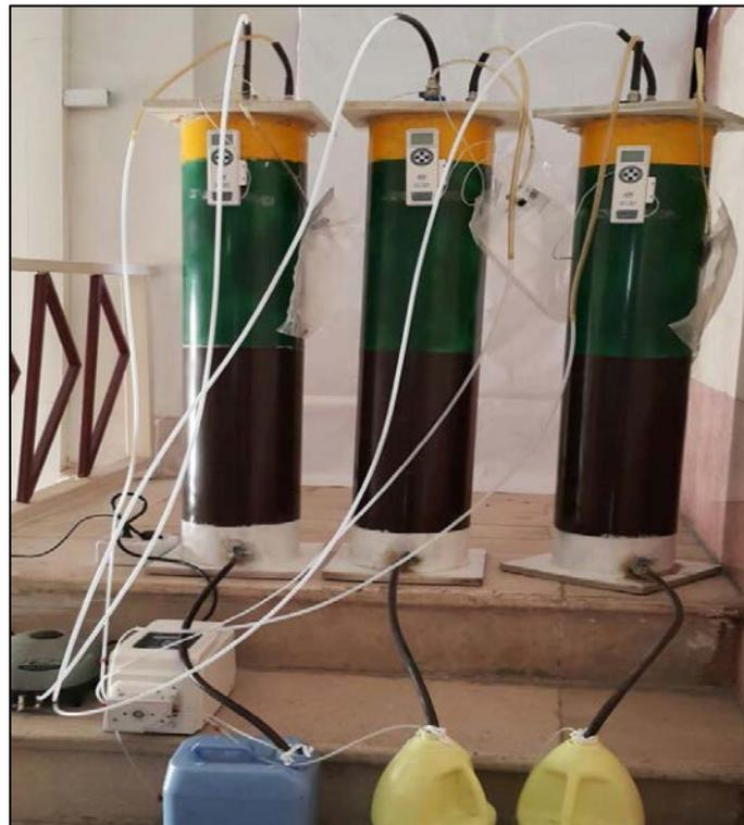
**Fig. 2.** Three lab-scale hybrids anaerobic –aerobic bioreactors with difference of operation conditions (R1, R2, and R3 bioreactors)
