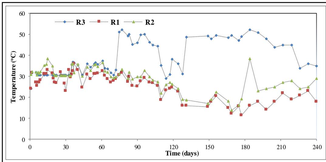
Fig. 4. The temperature profile of hybrid anaerobic-aerobic bioreactors during operation time for R1, R2, and R3 bioreactors
