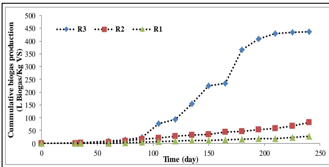
Fig. 5. The cumulative production of biogas with different operation conditions for R1, R2, and R3 hybrid anaerobic-aerobic bioreactors during 240 days of operation
