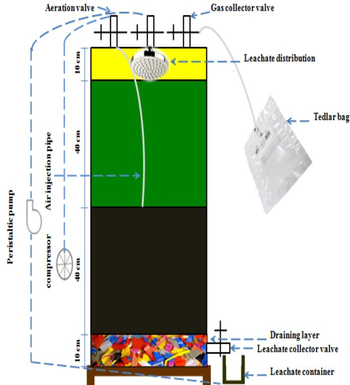
**Fig. 1.** Schematic image of a lab-scale hybrid anaerobic –aerobic bioreactor and its related accessories with 1 m in height and 20 cm in diameter (All three R1, R2, and R3 reactors are similar in appearance. (The dark brown and the green color represent the anaerobic and aerobic zones, respectively)
