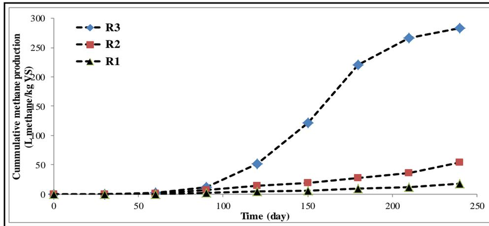
**Fig. 6.** The quantity of methane gas production in the three hybrid anaerobic–aerobic bioreactors with different operating conditions for R1, R2, and R3 reactors during 240 days of operation
