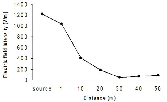
**Fig. 8.** Electric field intensity measured at the source and at the distances of 1, 10,20,30,40 and 50 m from 230 kV power substations
