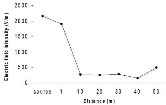
**Fig. 9.** Electric field intensity measured at the source and at the distances of 1, 10,20,30,40 and 50 m from 400 kV power substations
