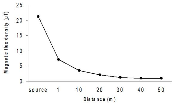
**Fig. 6.** Magnetic flux density measured at the source and at the distances of 1, 10,20,30,40 and 50 m from 400 kV power substations
