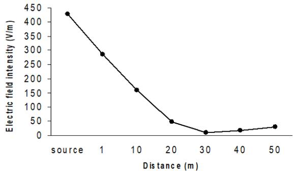
**Fig. 7.** Electric field intensity measured at the source and at the distances of 1, 10,20,30,40 and 50 m from 63 kV power substations
