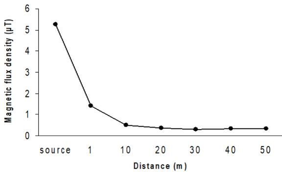
**Fig. 4.** Magnetic flux density measured at the source and at the distances of 1, 10,20,30,40 and 50 m from 63 kV power substations
