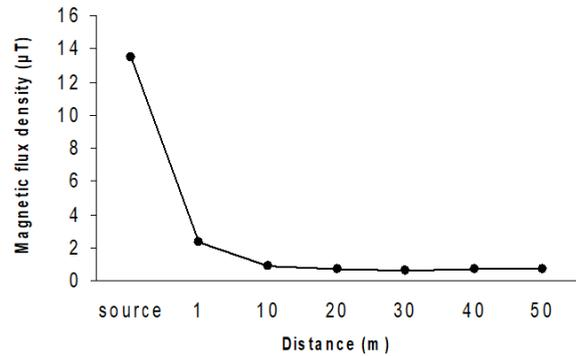
**Fig. 5.** Magnetic flux density measured at the source and at the distances of 1, 10,20,30,40 and 50 m from 230 kV power substations
