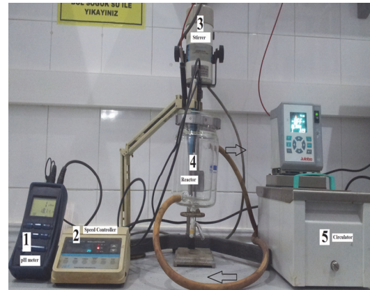
Fig. 1. Experimental set up (1. pH meter, 2. Speed controller, 3. Stirrer, 4. Reactor, 5. Circulator)
