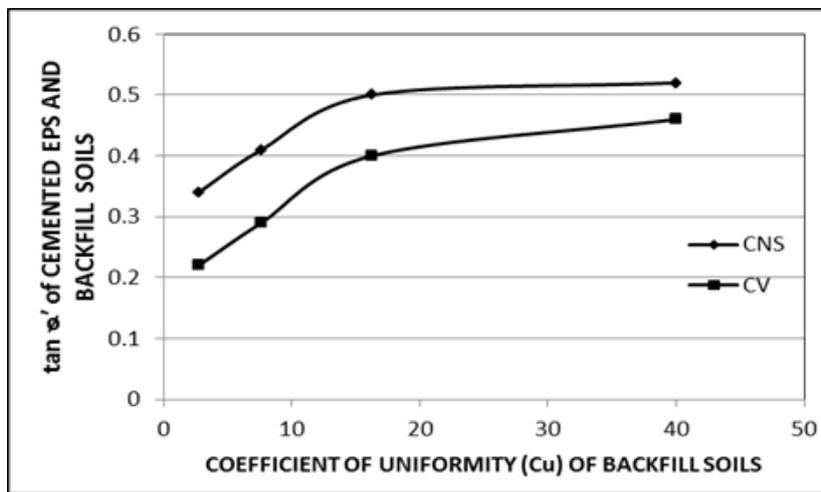
**Fig. 17.** Friction coefficient of light weight composites versus coefficient of curvature of the granular backfill
