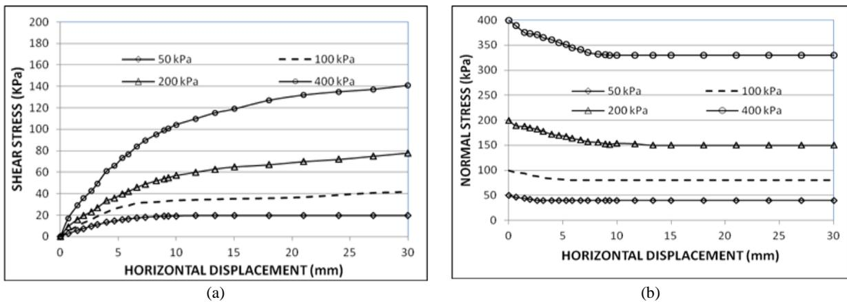
Fig. 10. CV stress and deformation curves for fine sand composite
