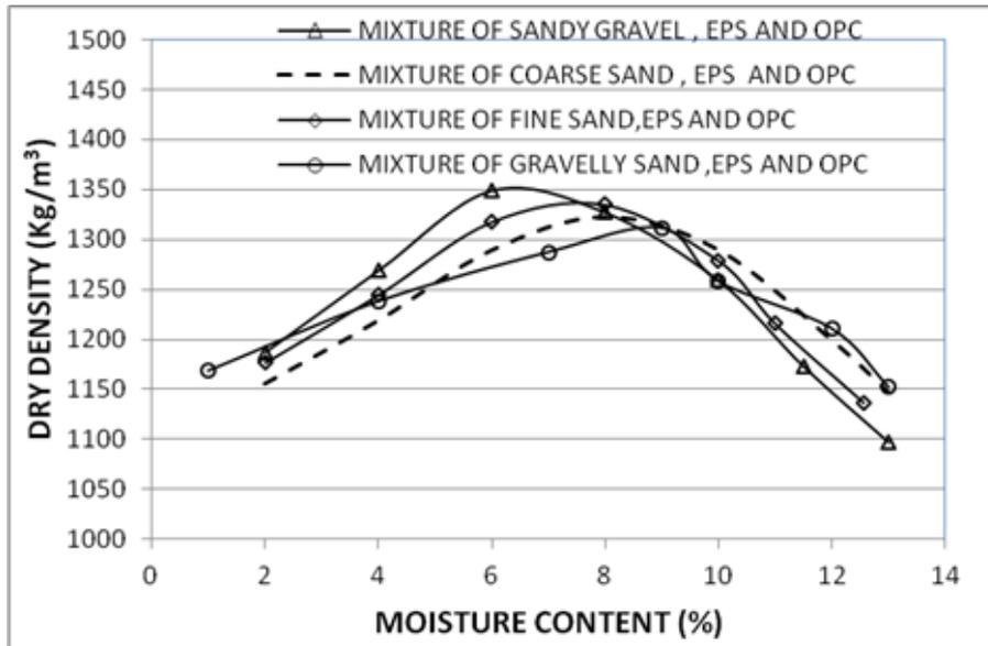
Fig. 5. Compaction curves of 3% cement stabilized backfill and EPS beads
