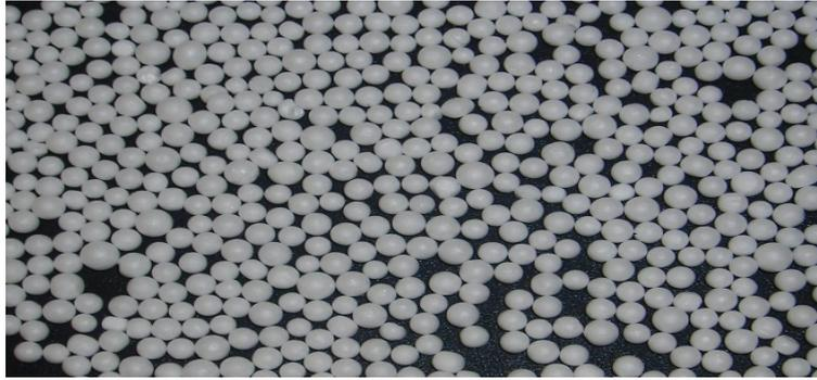
Fig. 1. Expanded polystyrene beads (EPS)
