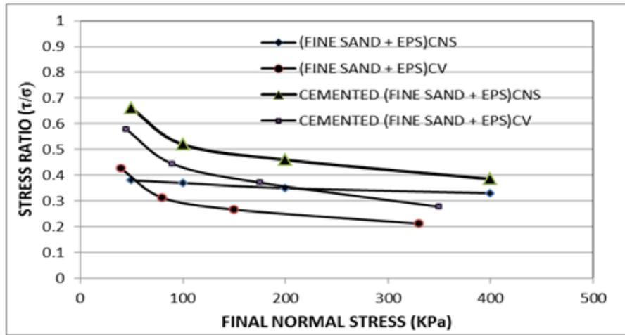
Fig. 15. The effect of initial normal stress on stress ratio of fine sand and cemented fine sand composite
