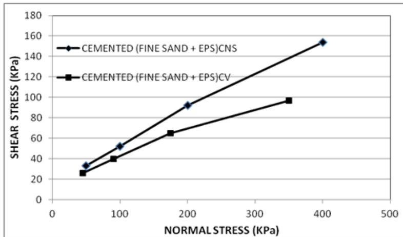
Fig. 14. CV strength envelopes for fine sand and cemented fine sand composite
