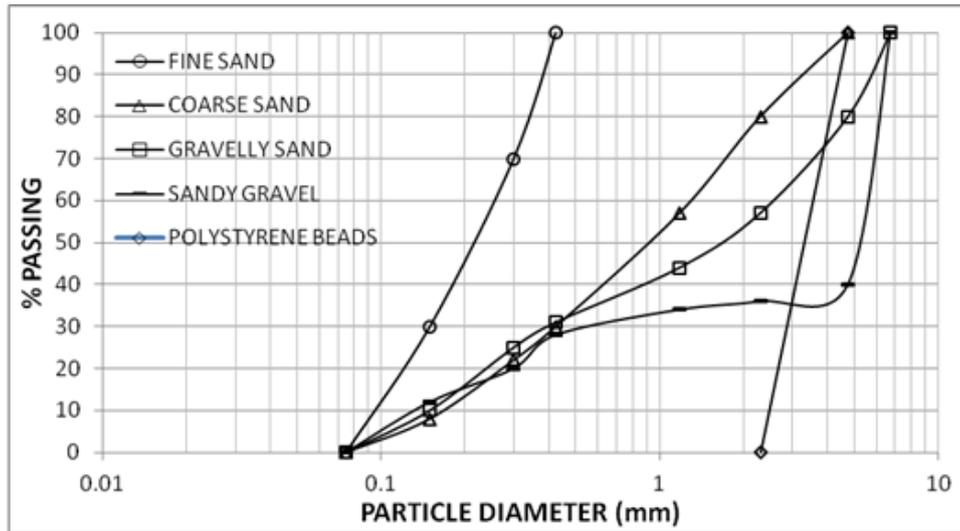
Fig. 2. Particle size distribution curves of granular backfill soils and EPS
