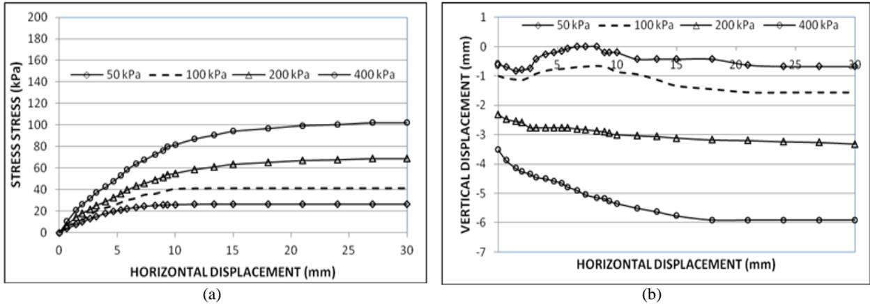
Fig. 12. CNS stress and deformation curves for cemented fine sand composite
