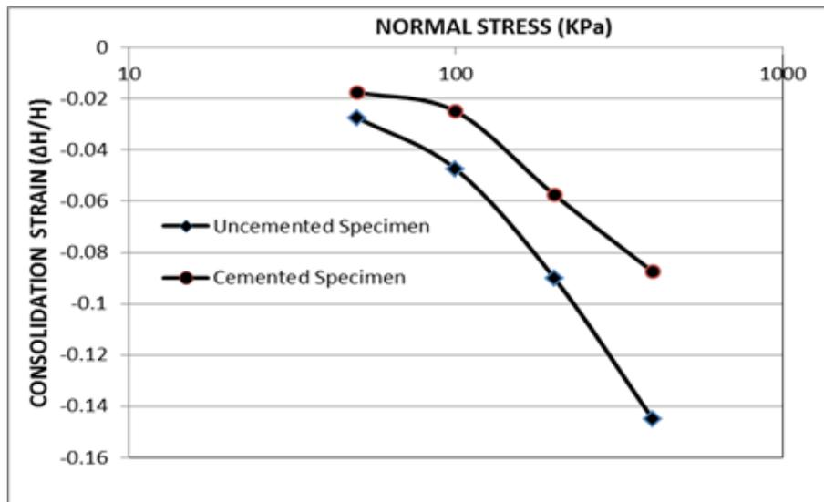
Fig. 16. The effect of normal stress on consolidation strain of cemented and uncemented fine sand composite for CNS tests
