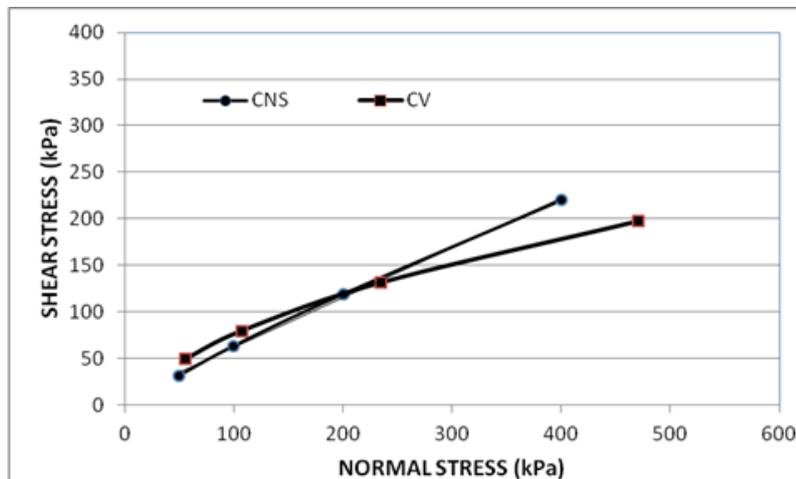
Fig. 8. CNS and CV strength envelope of fine sand
