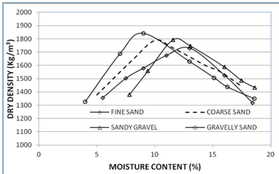
**Fig. 4.** Compaction curves for granular backfill materials
