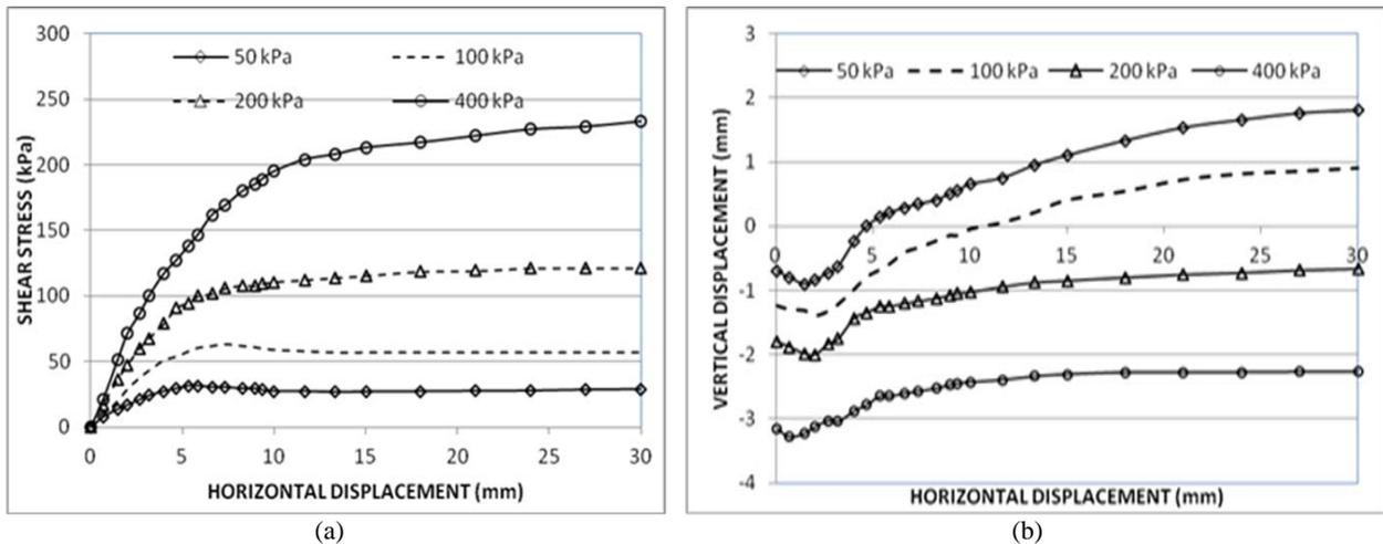
Fig. 6. CNS stress and deformation curves for fine sand
