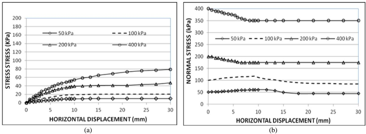
Fig. 13. CV stress and deformation curves for cemented fine sand composite
