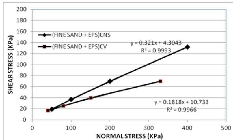
Fig. 11. CNS strength envelope for fine sand composite
