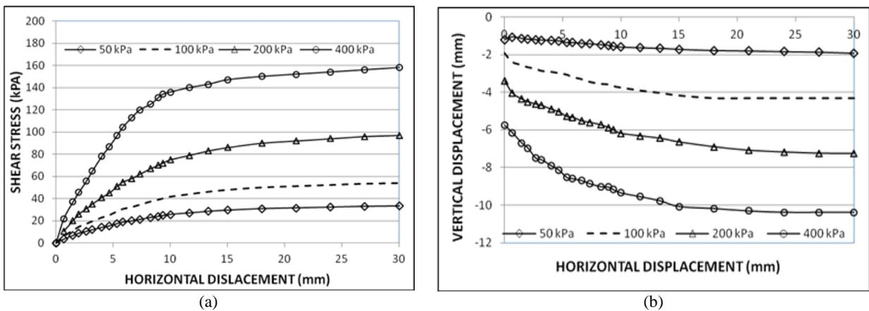
Fig. 9. CNS stress and deformation curves for fine sand composite
