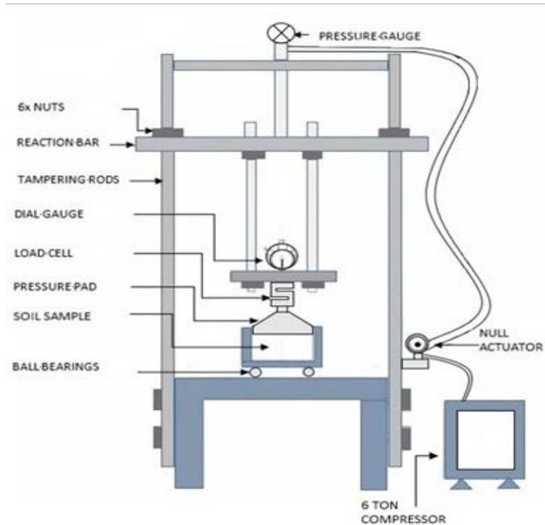
Fig. 3. Direct shear apparatus with constant volume frame
