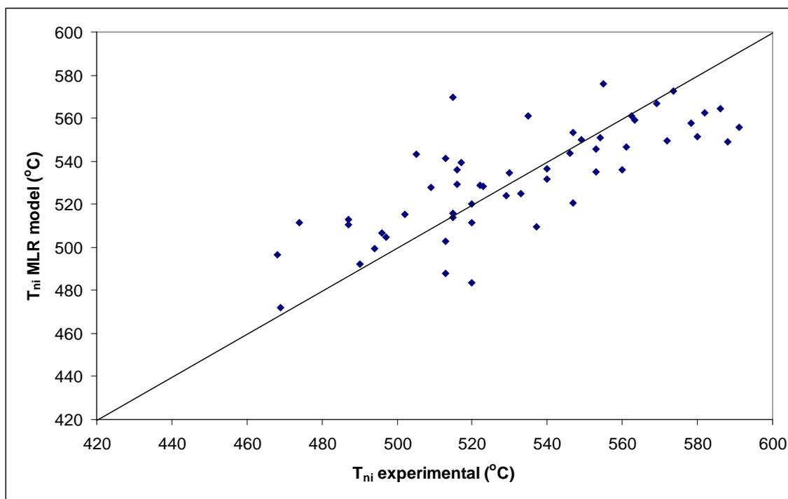
**Fig. 1.** Comparing the experimental values with those calculated using the MLR model for the temperature at which, following the degradation process, 10% of the initial amount of the sample subjected to analysis under an inert atmosphere of  $N_2$  ( $T_{ni}$ ) is lost
