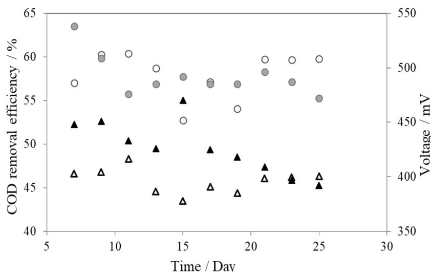
**Fig. 5.** COD removal efficiency (open) and voltage generation across the 100  $\Omega$  resistance (closed) of PEM-MFC (circles) and EP-MFC (triangles) as a function of time during continuous feed of MFCs (commenced at day 7)
