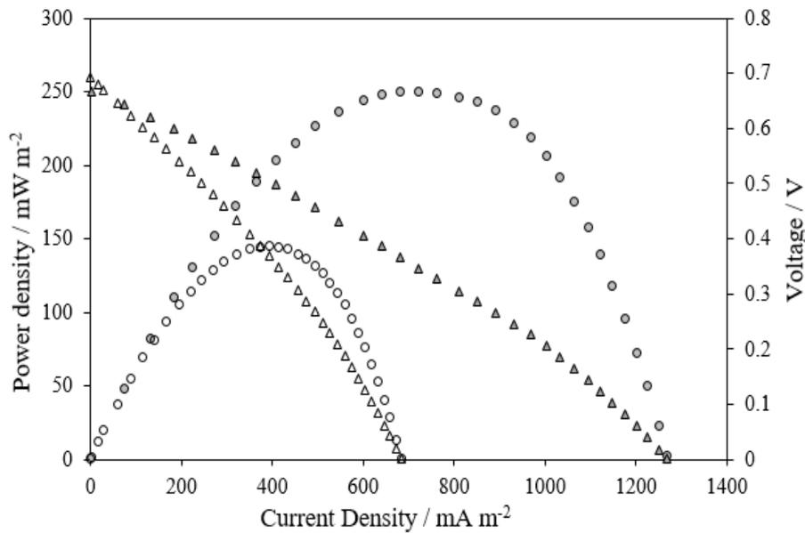
Fig. 6. In-situ polarization curves, recorded on day 25, cell voltage and power density versus current density for PEM (grey closed) and earthen plate (black open) MFCs
