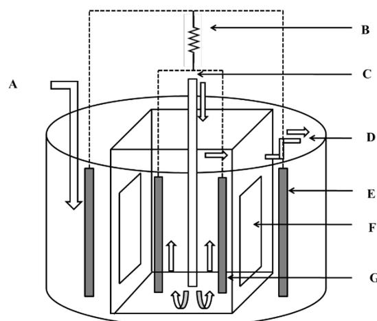
**Fig. 1.** Schematic diagram of the MFCs used in the study: (A)  $K_3Fe(CN)_6$  catholyte (B) external resistance load (C) cell culture medium anolyte (D) anolyte influent (E) catholyte effluent (F) membrane (G) anode
