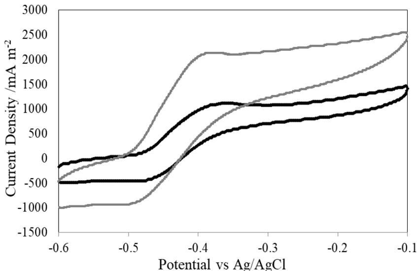
Fig. 3. Cyclic voltammograms (1 mV/s) of anodic biofilm, recorded in-situ on the 19th day of operation of the cells under 100 Ω external resistors, for the PEM-MFC (grey) and EP-MFC (black) systems
