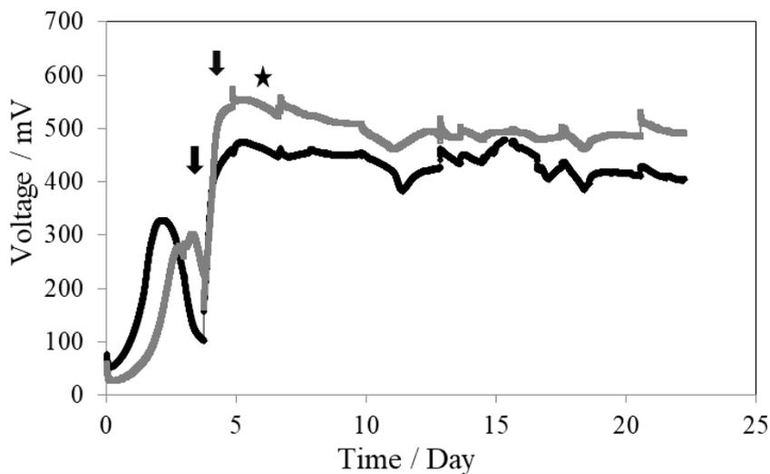
Fig. 2. Voltage generations as a function of time for the PEM-MFC (grey) and the EP-MFC (black). Arrows indicate replacement with fresh feed and star indicates the time when the reactors were switched from batch to continuous mode operation
