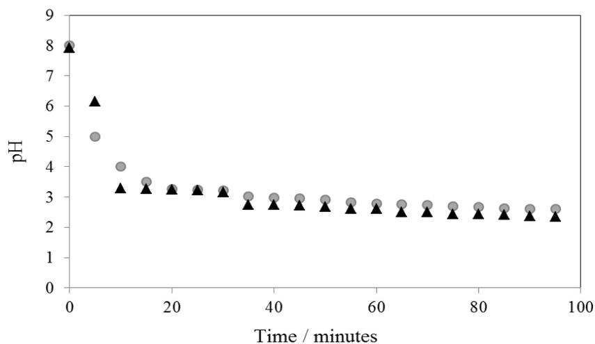
**Fig. 4.** A comparison of the change in pH of the catholyte chamber, initially containing distilled deionized water, as a function of time upon introduction of 1 M sulphuric acid into the anolyte chamber for PEM (grey circles) and earthen plate (black triangles) MFCs
