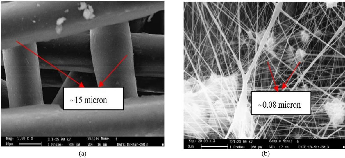
**Fig. 4.** Surface microstructure of new (a) filter medium A and (b) filter medium B
