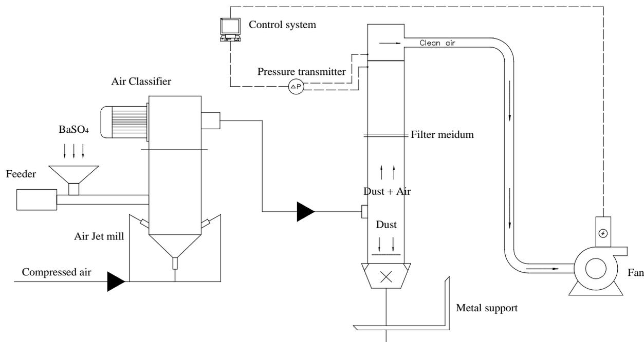
**Fig. 1.** Experimental process of first-used filter media
