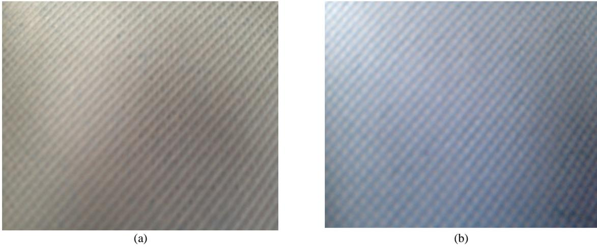
**Fig. 3.** Apparently similar fabrics of (a) filter medium A and (b) filter medium B
