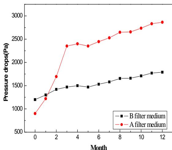
**Fig. 12.** Pressure drops of A and B filter media via time
