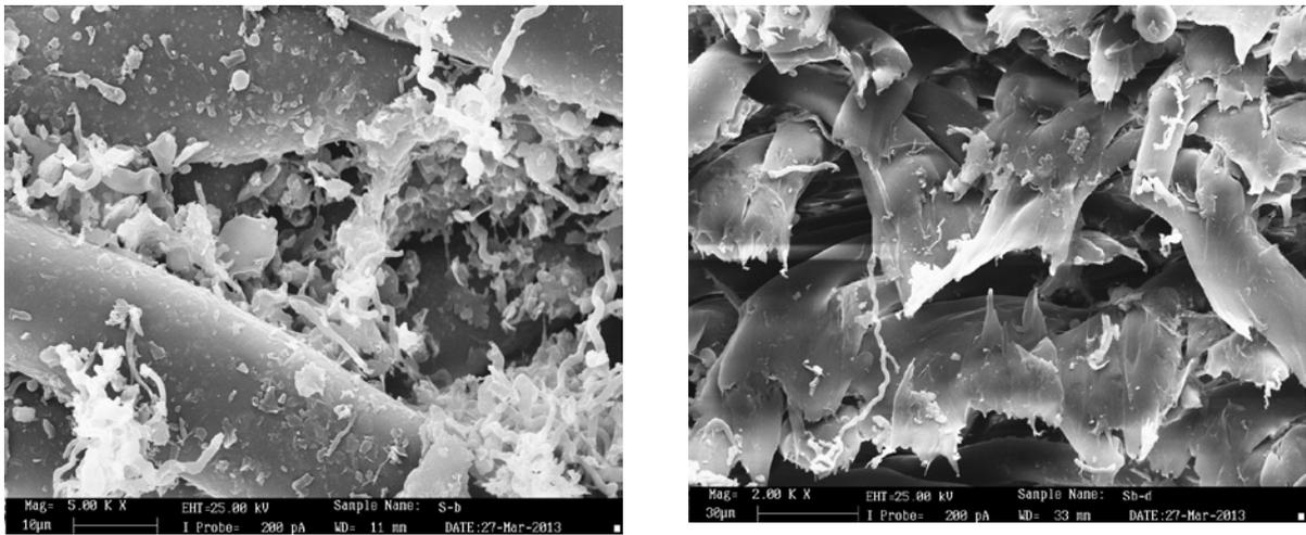
**Fig. 10.** Filtration behaviors of filter media B with one year used: (a) surface of filter medium B with one year, (b) cross section of filter medium B with one year
