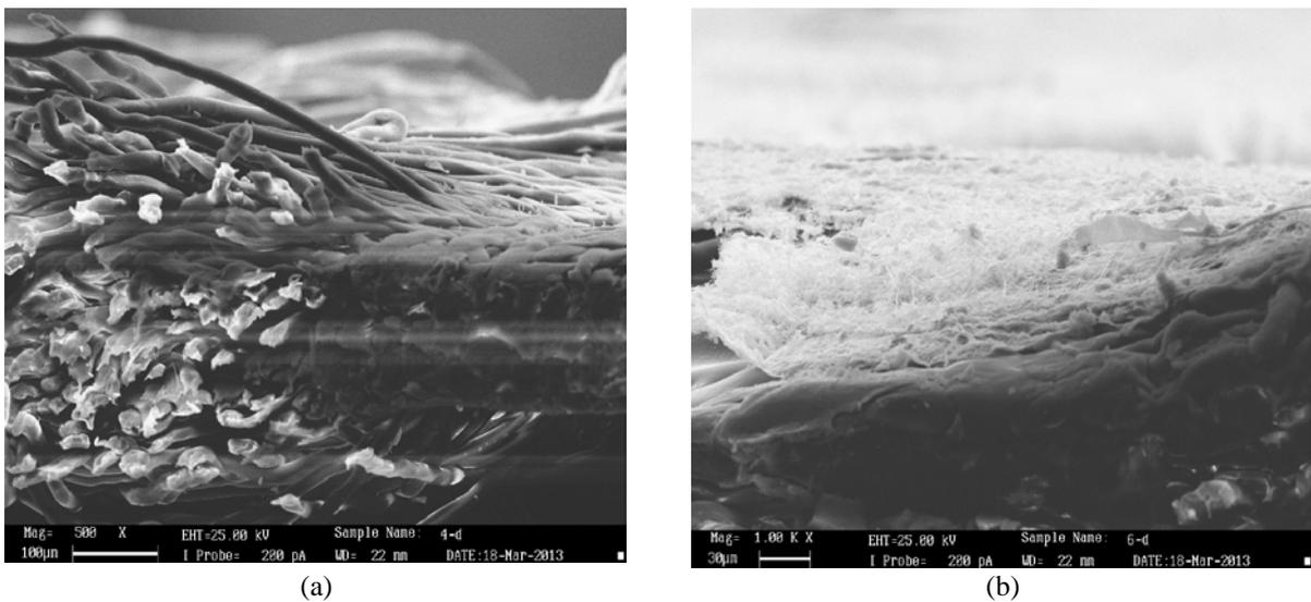
**Fig. 5.** Cross section microstructure of new A and B filter media: (a) filter medium A and (b) filter medium B
