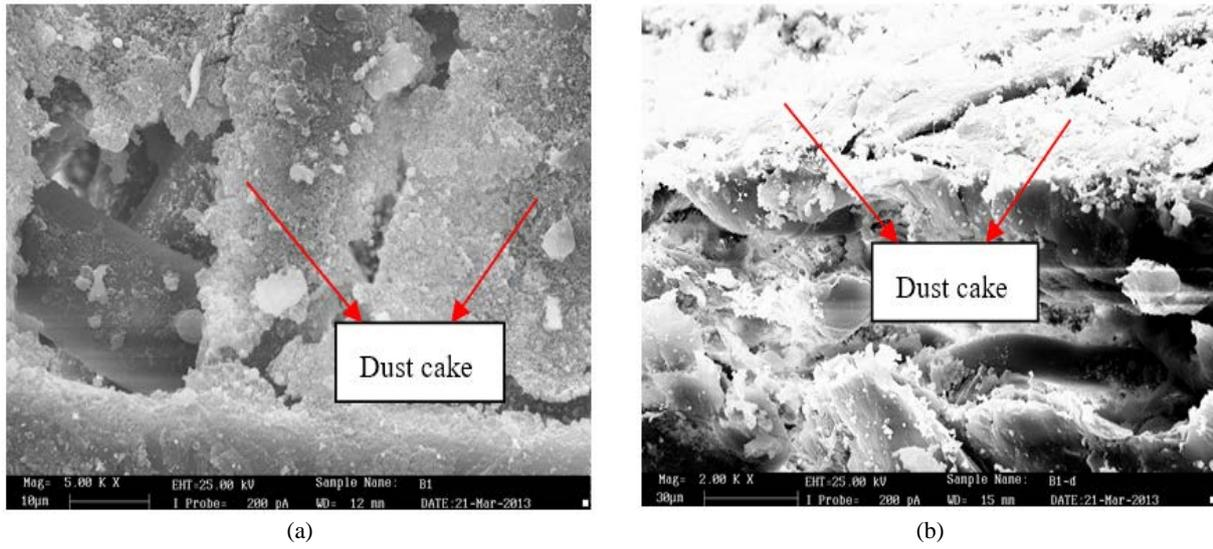
**Fig. 9.** Filtration behaviors of filter media A with one year used: (a) surface of filter medium A with one year, (b) cross section of filter medium A with one year
