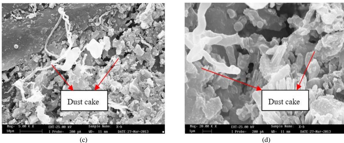
**Fig. 11.** Dust cake effect: (a) photo of B filter medium, (b) 1000 x of B filter medium, (c) 5000 x of B filter medium, (d) 20000 x of B filter medium
