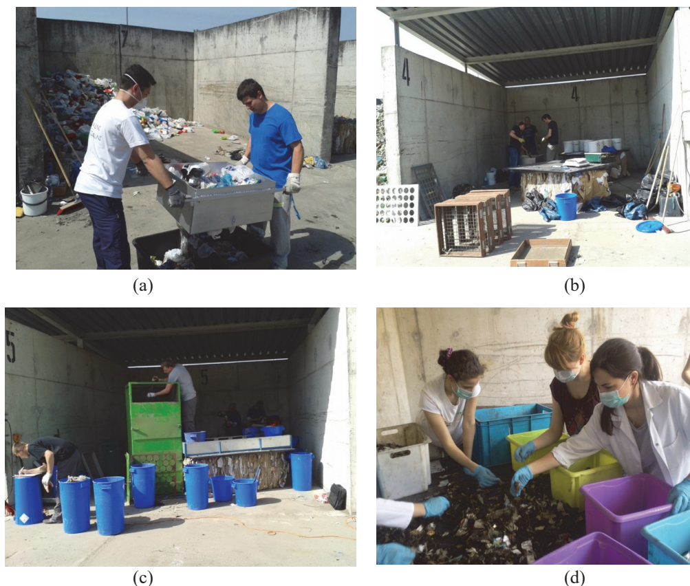
Fig. 2. Sorting by different teams: (a) represents manual sieving procedure, (b) - typical manual sieves, (c) - vibrating sorting machine, (d) - manual determination of material composition
