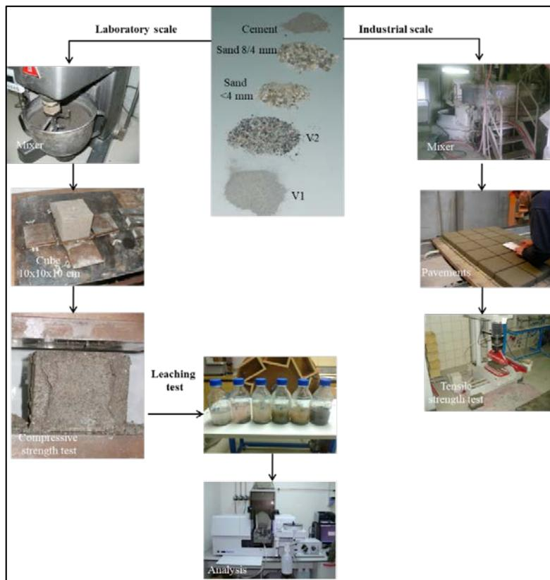
Fig. 3. Carried out procedures on experimental concrete samples
