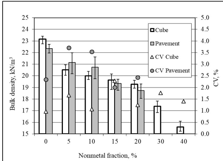
Fig. 6. Volume weights of specimens
