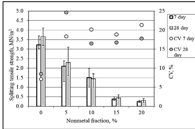
Fig. 5. Tensile strengths of pavements  $f_{ct,sp}$
