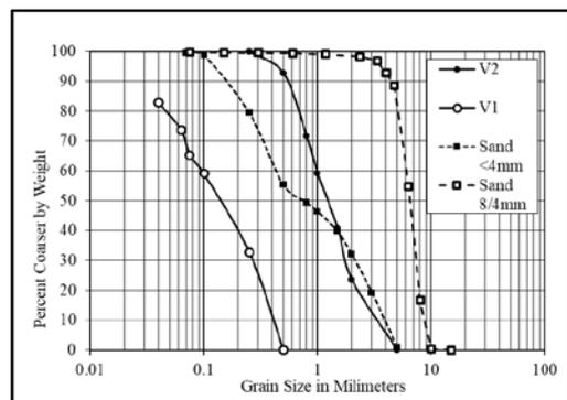
Fig. 1. Size distribution of NMF and mineral filler samples
