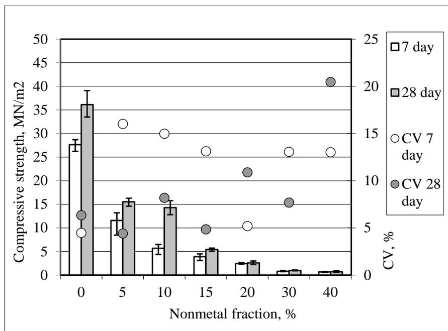
Fig. 4. Results of compressive strengths analysis of specimens
