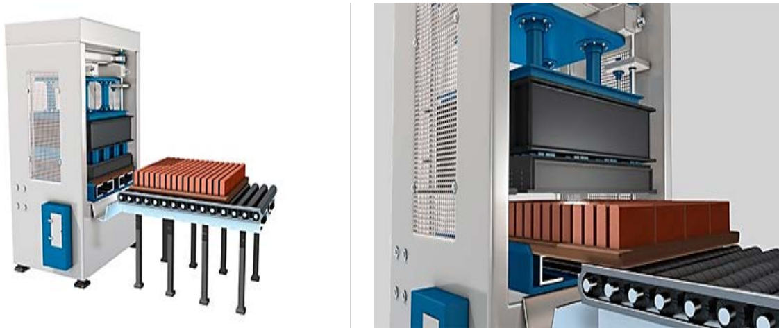
Fig. 3. High compression press used for the production of the “Ri-block®”
