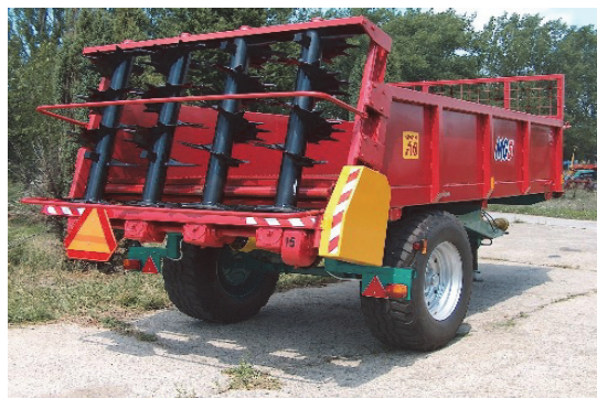
Fig. 1. (a) Spreading apparatus of machine MG5; (b) Spreading machine MG5: 1) axis; 2) helical coil; 3) disk; 4) blade
