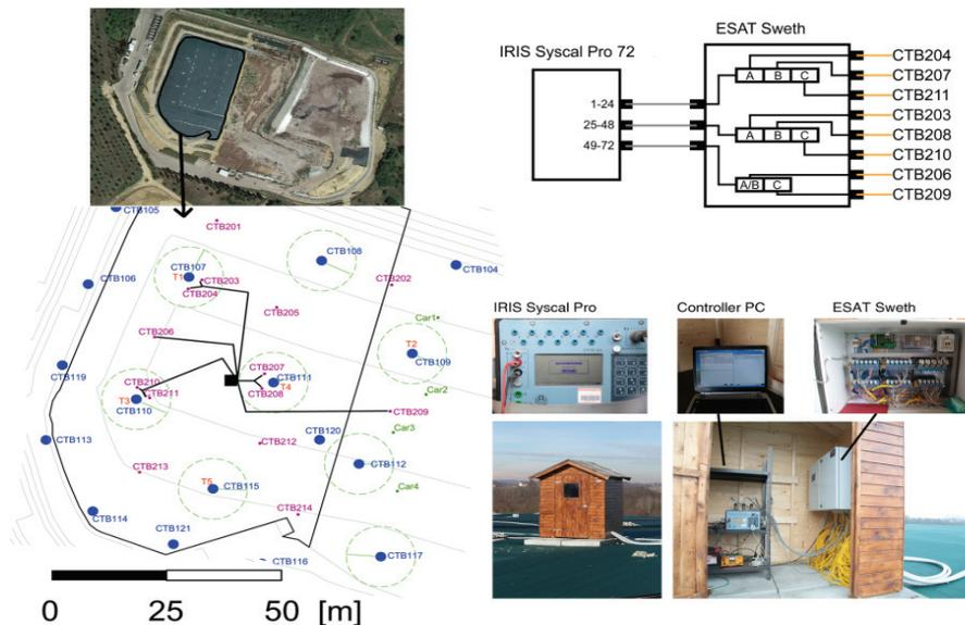
**Fig. 4.** Map of the cell after the disposal of the final coverage; the black lines on the map refer to the electrical connection between the boreholes (equipped with geophysical sensors) and the remote monitoring system (in the centre of the cell). The acquisition unit (Iris Syscal Pro) is connected to the boreholes through a multiplexer (Esat Sweth); an external PC guarantees the remote control of the unit)
