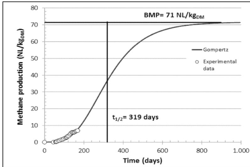
Fig. 6. Cumulative methane yield in the tested lysimeter
