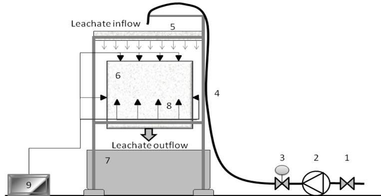
**Fig. 8.** Experimental set up of a single cube of pretreated waste for the small-scale re-circulation test and resistivity monitoring: 1) closure valve, 2) pump, 3) regulator valve, 4) delivery pipe, 5) distribution grid, 6) waste, 7) collecting tank (discharge), 8) electrodes, 9) acquisition unit for resistivity monitoring
