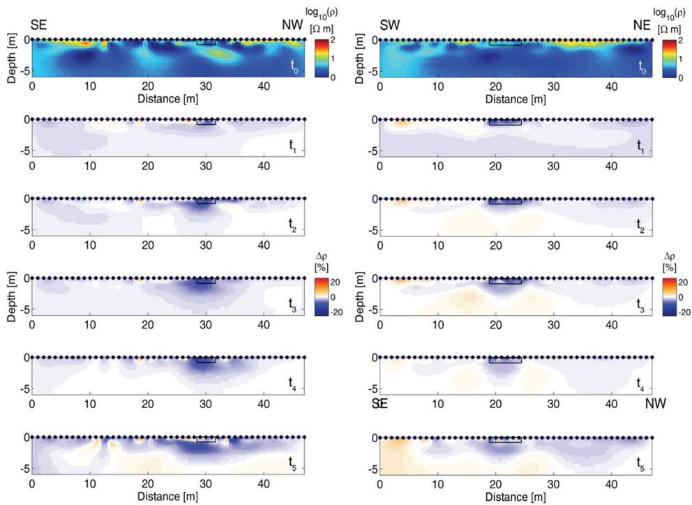
**Fig. 11.** Relative differences obtained by inversion of resistance data at time-lapse steps (compared to the corresponding background data); the experiment refers to an infiltration test of 6 m<sup>3</sup> of water, infiltrated from the top of the landfill
