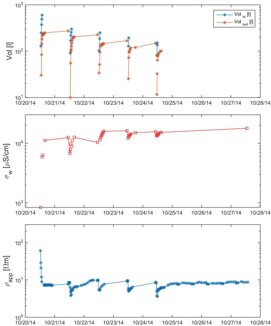
**Fig. 9.** “Cube-scale” test: in-flow and out-flow volumes (top); fluid conductivity of the recirculated fluid (center); apparent resistivity measured with the quadripole at the top of the cube (bottom)
