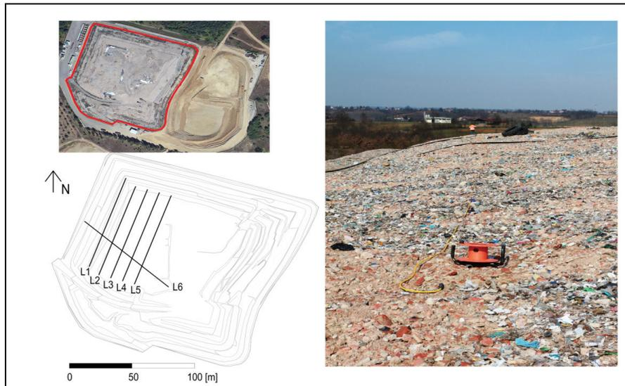
**Fig. 1.** Plan view of the landfill and position of geophysical profiles for waste characterization (the three images are the location of the vertical boreholes equipped with electrodes for geophysical monitoring)
