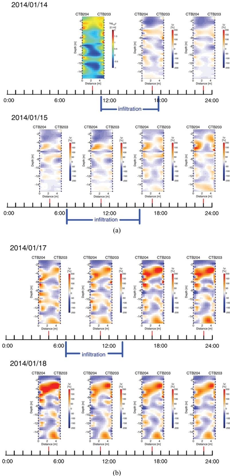
**Fig. 13.** Time-lapse geo-electrical monitoring of a pilot re-circulation test, at boreholes CTB203-CTB204: (a) background resistivity image and first two days of infiltration; (b) end of the infiltration and redistribution phase
