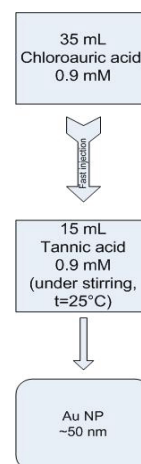
Fig. 1. Schematic representation of gold nanoparticles synthesis, sample A3
