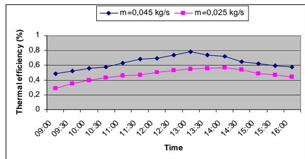
**Fig. 6.** Thermal efficiency variation in time for different air mass flow rates
