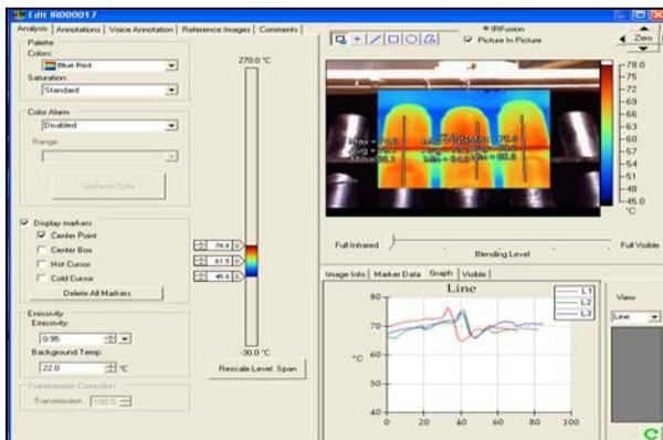
Fig. 9. Visualization of temperature variation on absorber surface in area of support elements
