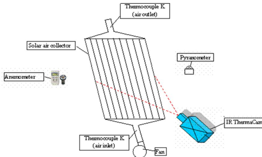
Fig. 1. Schematic view of experimental set-up
