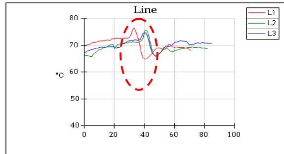
Fig. 10. Temperature variation on absorber surface due to heat loss by conduction
