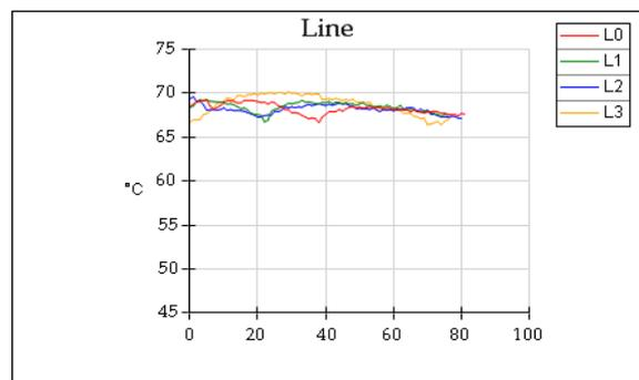
Fig. 12. Visualisation of temperature variation on surface of lateral tubes
