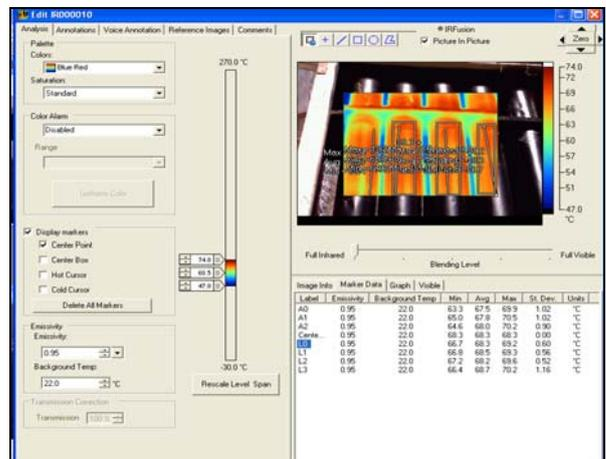
Fig. 11. Visualisation of temperature variation on absorber surface for lateral tubes
