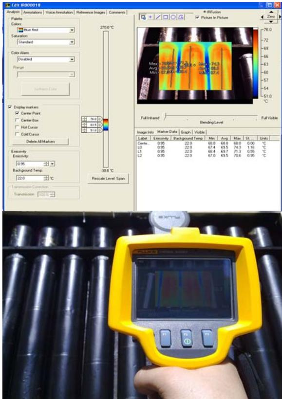
Fig. 7. Temperature measure on the absorber surface with FLIR Fluke Ti10 Thermal Imager W/IR Fusion
