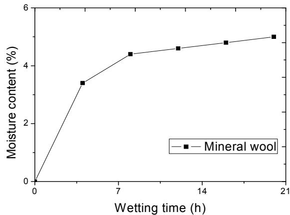
Fig. 2. The adsorbed amount of water as a function of the wetting time at 90% relative humidity for the mineral wool sample
