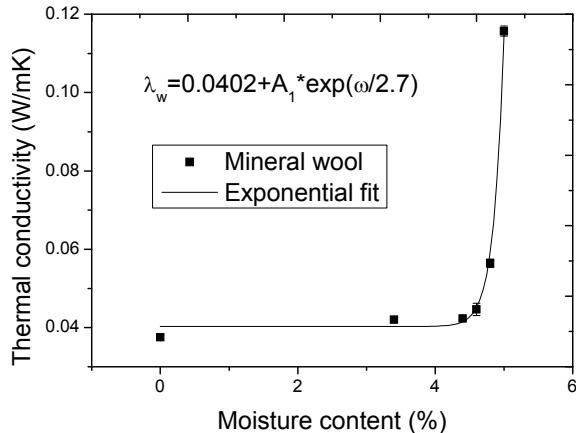
Fig. 1. The thermal conductivity of the mineral wool sample as a function of the moisture content
