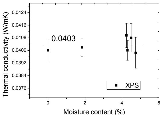
**Fig. 7.** The thermal conductivity of the XPS as a function of the moisture content
