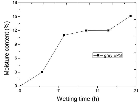
**Fig. 6.** The adsorbed amount of water as a function of wetting time at 90% relative humidity for the grey EPS
