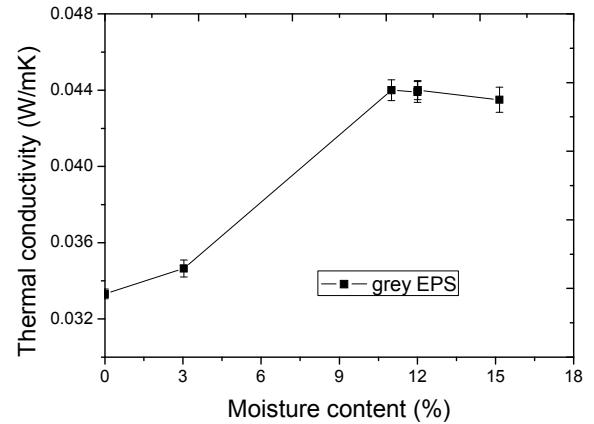
**Fig. 5.** The thermal conductivity of the grey EPS sample as a function of the moisture content
