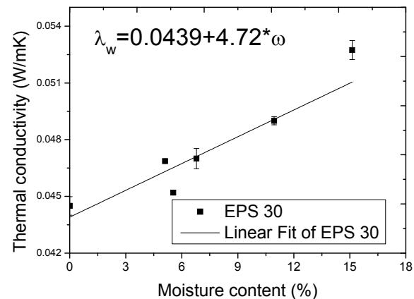
Fig. 3. The thermal conductivity of the EPS 30 as a function of the moisture content
