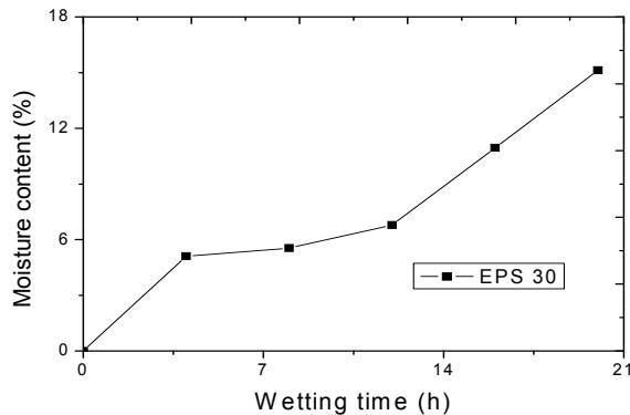
**Fig. 4.** The adsorbed amount of water as a function of the wetting time at 90% relative humidity for the EPS 30
