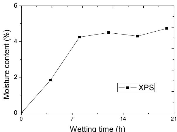
**Fig. 8.** The adsorbed amount of water as a function of the wetting time at 9% relative humidity for the XPS
