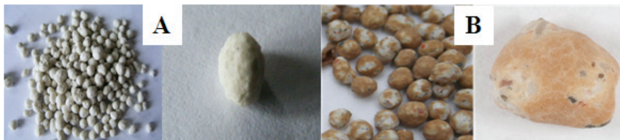
Fig. 1. A - granules of the starting material - commercial, multicomponent fertilizer ( s0 ), B - granules of the fertilizer covered with the layer of chitosan - mass ratio chitosan/fertilizer 8/100 ( s1 )
