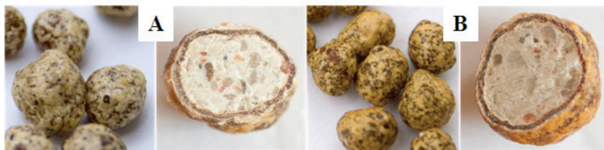
Fig. 4. Granules of the fertilizer covered with the mixture of chitosan, natural wax, glycerine and sodium tripolyphosphate after two steps (A) and after the third step (B) of the process
