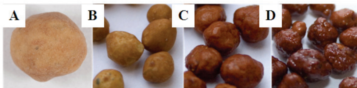
Fig. 3. Granules of the fertilizer covered with the mixture of chitosan, natural wax and glycerine with various mass ratios of chitosan to fertilizer: A - 8/100 (s5), B - 12/100 (s6), C - 18/100 (s7) and D - 24/100 (s8)
